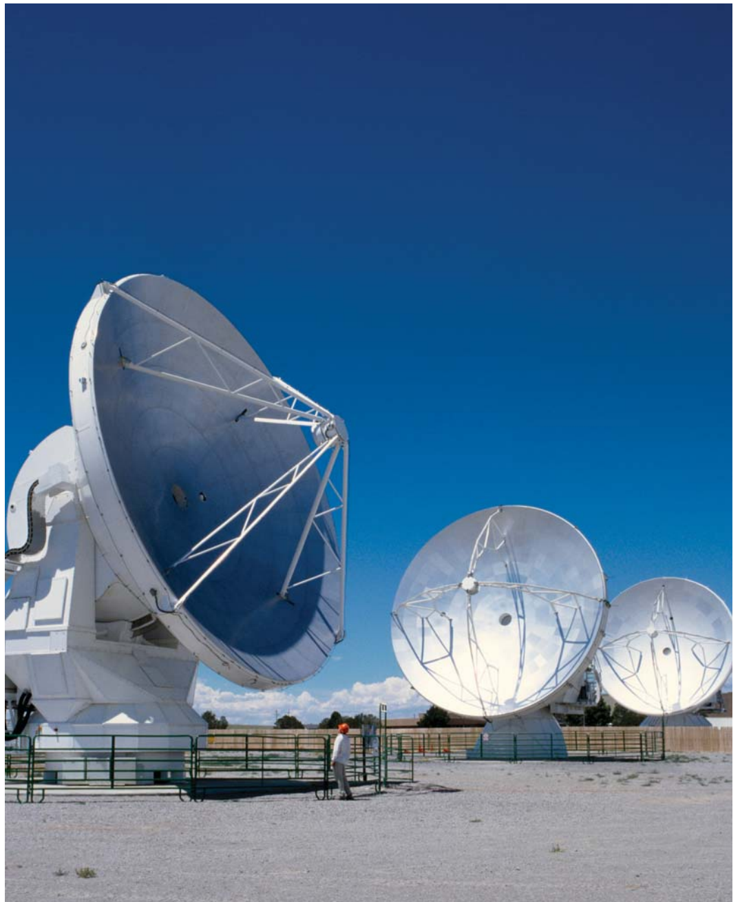
The prototype ALMA antennas deployed by Alcatel, VertexRSI, and Mitsubishi (left to right) at the ALMA Test Facility in New Mexico. Each of these antennas has been designed to meet ALMA's exacting technical specifications, and will have 10 – 100 times more sensitivity and angular resolution than current millimeter wavelength telescopes. Credit: NRAO/AUI
