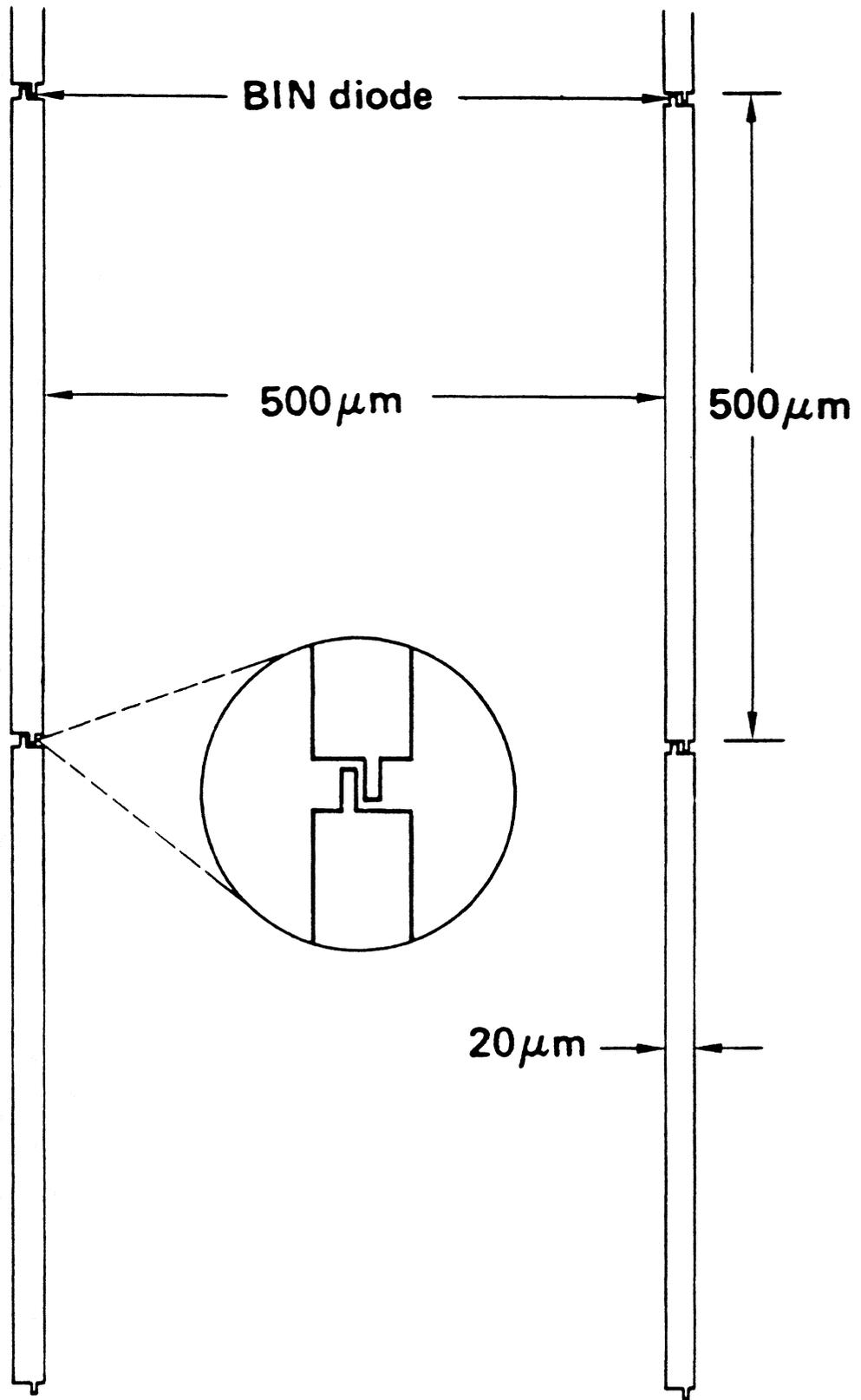
Figure 6. Metal grid design for BIN diode tripler.
