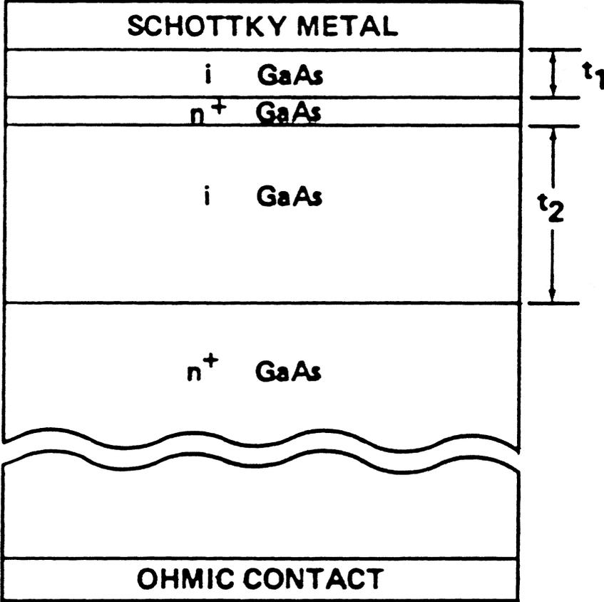
Figure 5. Structure of the GaAs BIN diode.
