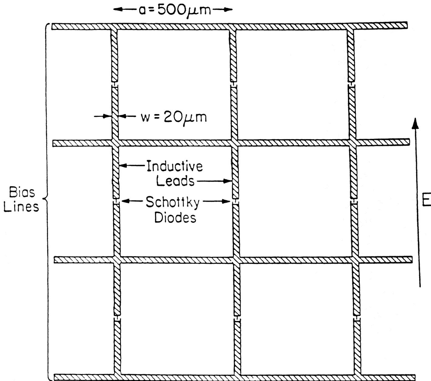
Figure 1. Metal grid design for Schottky diode doubler.
