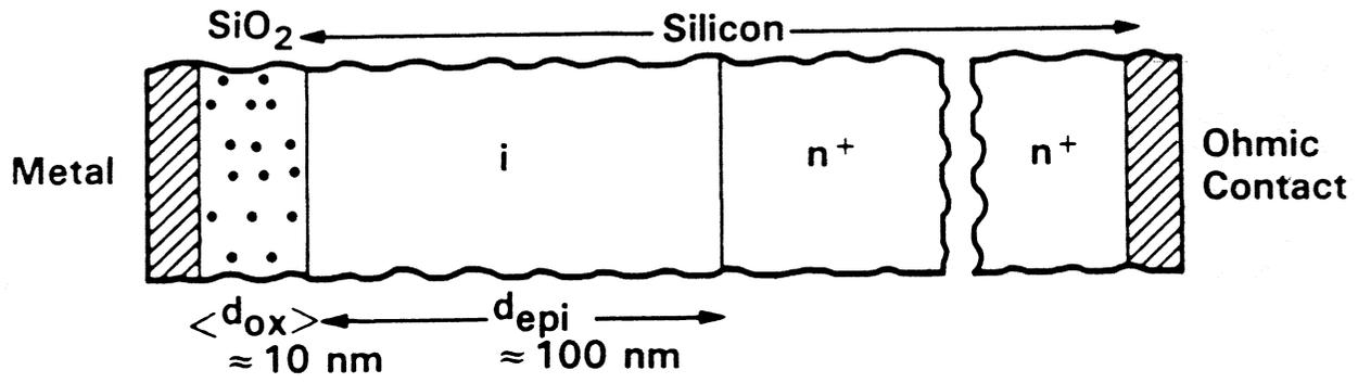
Figure 3. Structure of the thin MOS diode.
