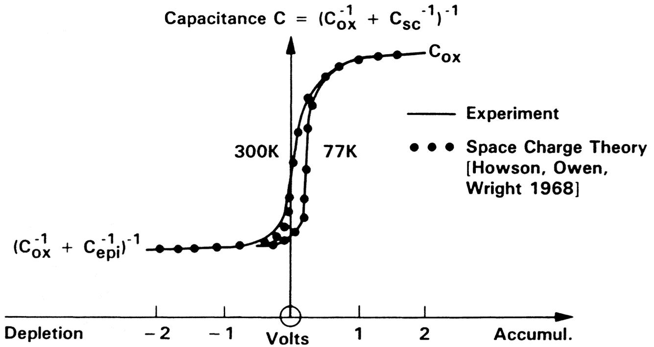
Figure 4. Capacitance-voltage characteristic from the thin MOS diode.
