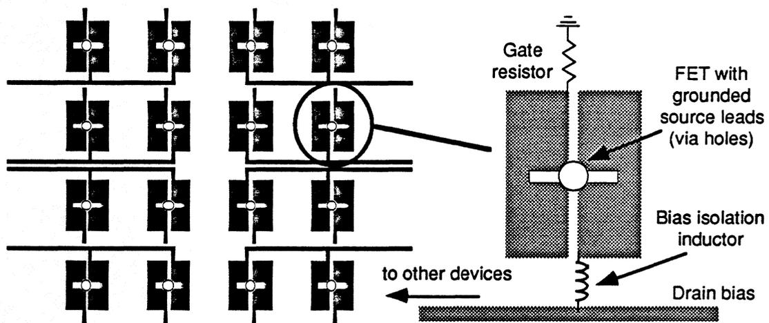
**Figure 3** — Sketch of the array which uses Fujitsu fsx02 MESFETs, showing bias arrangement and individual element design. Elements measure 11 mm by 15 mm and the spacing of the elements is  $0.67 \lambda_0$  between centers. The bias inductor reduces element interactions along the bias line.
