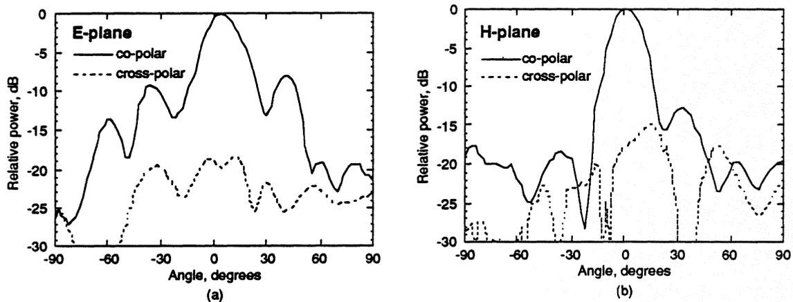
**Figure 4** — (a) E-plane and (b) H-plane patterns for the  $4 \times 4$  MESFET array. The measurements were made at 8.27 GHz, using a flat, 2.5 cm thick dielectric reflector with a dielectric constant of 4. The good patterns indicate in-phase operation.
