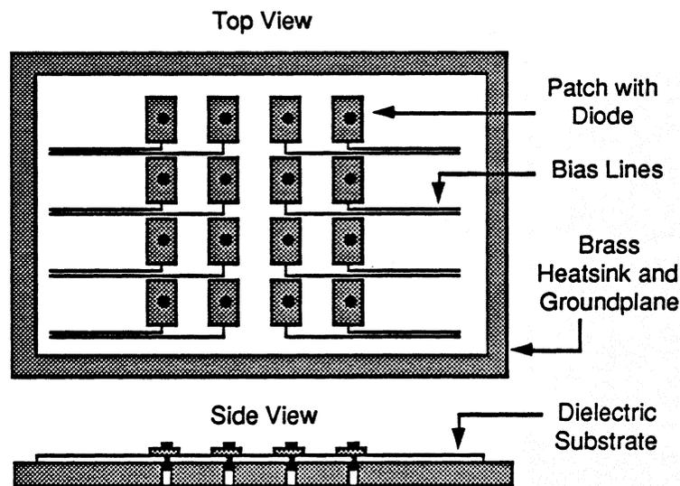
**Figure 1** — Diagram of Gunn diodes mounted into a 4×4 array of microstrip patches. The brass block serves as a groundplane, heatsink, and DC bias return. Individual bias to each element is applied at an RF null.
