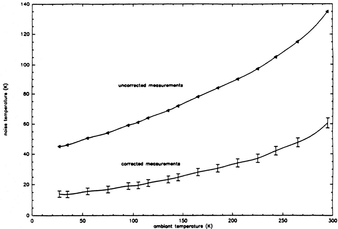
Fig. 10 : Noise temperature function of physical temperature
