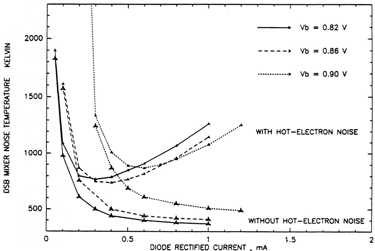
Fig. 2 : Computed minimum DSB mixer noise temperature versus  $P_{OL}$ , with and without hot-electron noise.
