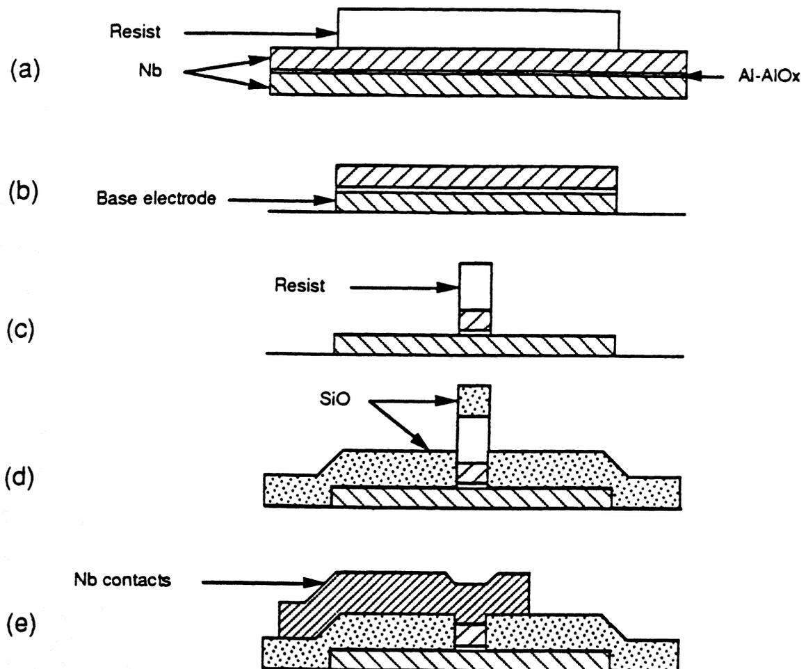
*Fig. 11 : Fabrication process of Nb/Al-AlOx/Nb junctions (a) Nb/Al-AlOx/Nb deposition. Definition of the base electrode by photolithography. (b) Trilayer etching. (c) Upper electrode etching. (d) self aligned deposition of a SiO<sub>2</sub> insulating layer. (e) Nb interconnection layer.*
