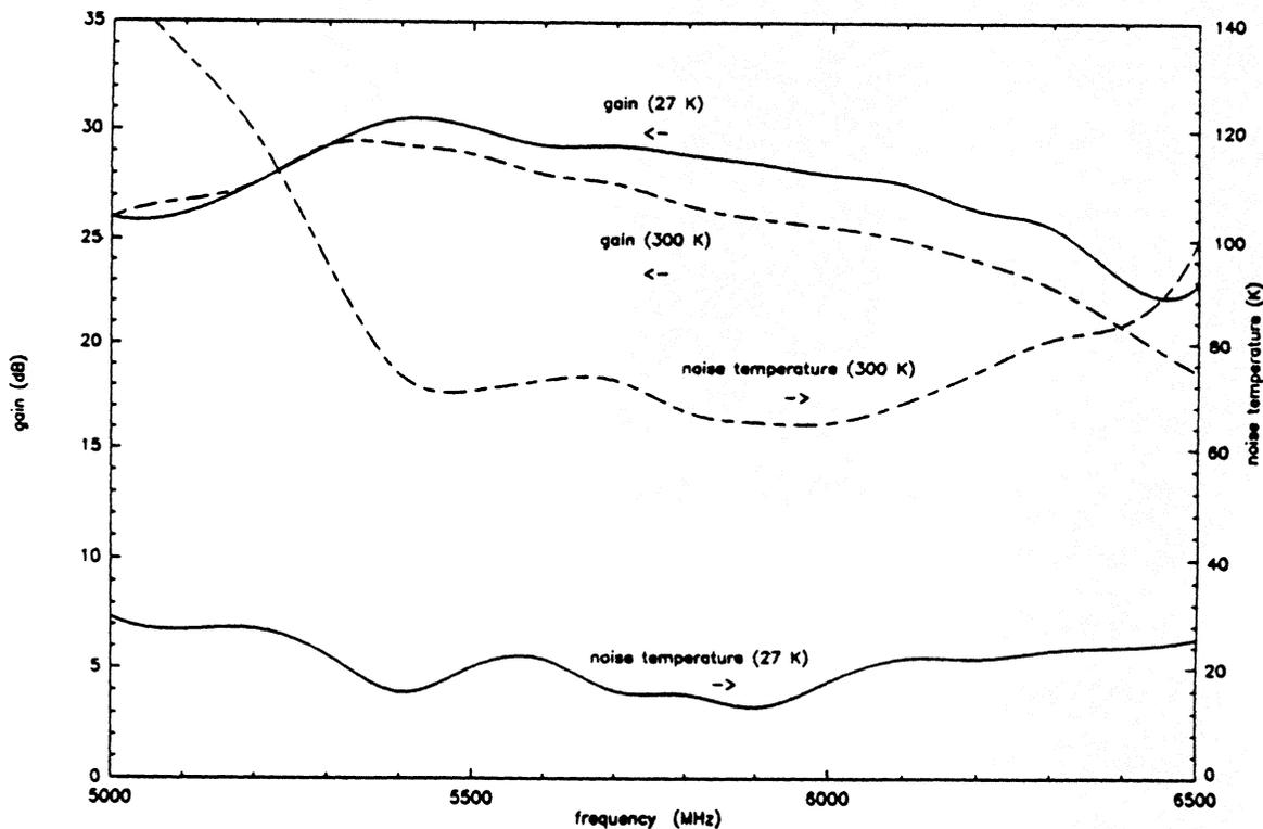
Fig. 9 : Measured characteristics of the amplifier
