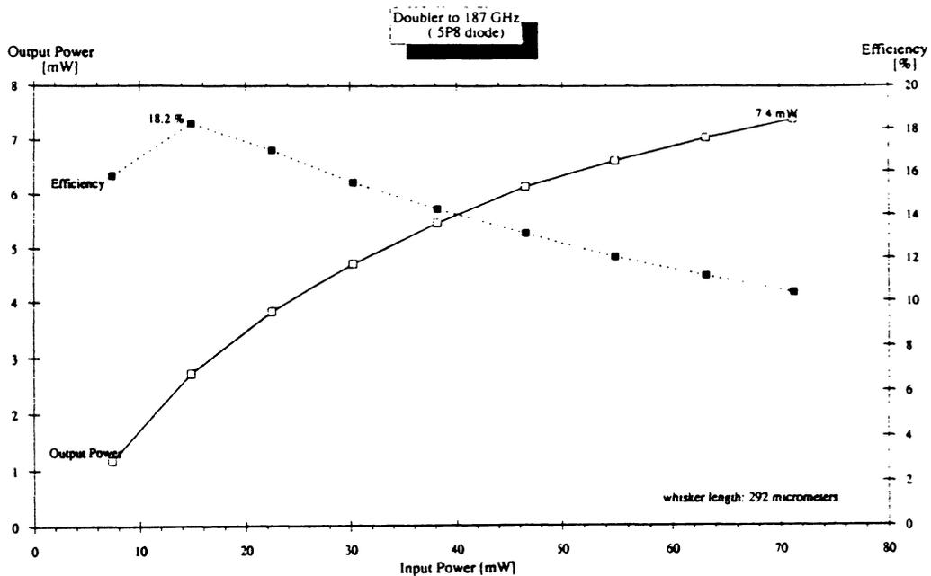
The second 187/374 GHz doubler, designed with an integrated horn (Fig. 7a) using U. Va varactor is under tests at this moment. The output power (Fig. 7b) is not quite powerful enough to drive a Schottky mixer ; but it is enough to pump an SIS junction.
