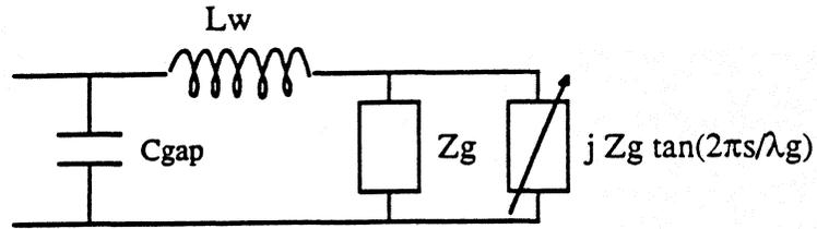
Fig. 3 : Simplified embedding network at fundamental frequency
