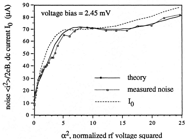
**Figure 6** Photon-induced noise in the single Hypres SIS junction as a function of the normalized rf voltage squared. The junction was biased on the first photon step at 2.45 mV. Also shown is the measured dc current for comparison to shot noise.
