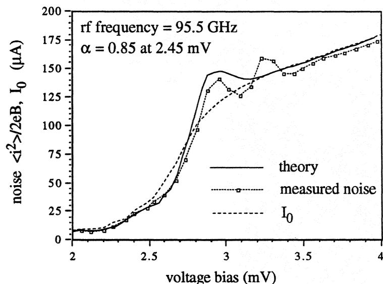
**Figure 5** Photon-induced noise in a single Hypres junction as a function of dc bias voltage. The theory is calculated from Tucker's theory, including the contribution from vacuum noise. Also plotted is the measured dc current  $I_0$  which includes the photon induced current. The dc IV curve, with no incident radiation, for this junction is shown in figure 3(b).
