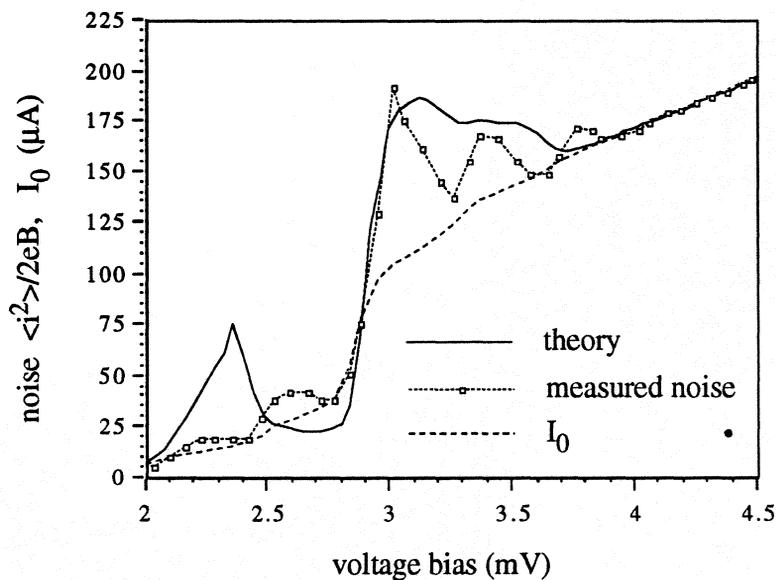
**Figure 9** Photon noise in single IBM junction as a function of the voltage bias. The rf power corresponded to  $\alpha = 1.10$  at 2.68 mV. The rf frequency is 95.5 GHz. Also plotted is the measured dc current, for comparison to shot noise.
