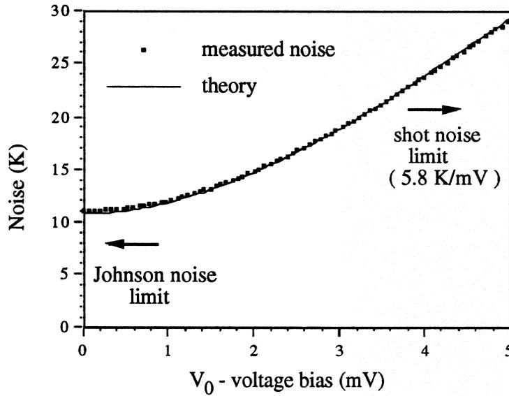
**Figure 2** Measured and theoretical noise for a single niobium tunnel junction in its NIN state at a temperature of 10.79 K. The theory is calculated from the fluctuation dissipation relation of equation 4.
