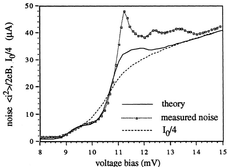
**Figure 7** Photon induced noise in a four junction series array as a function of the bias voltage. Also plotted is the measured dc current divided by the number of junctions in the array, for comparison to shot noise. The rf power power corresponds to  $\alpha = 1.0$  at 9.87 mV and rf frequency is 95.5 GHz.
