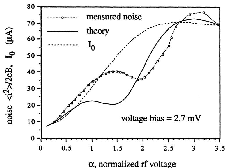
**Figure 10** Photon induced noise in the single IBM junction as a function of normalized rf voltage. The junction was biased on the first step at 2.7 mV. Also shown is the measured dc current, for comparison to shot noise.
