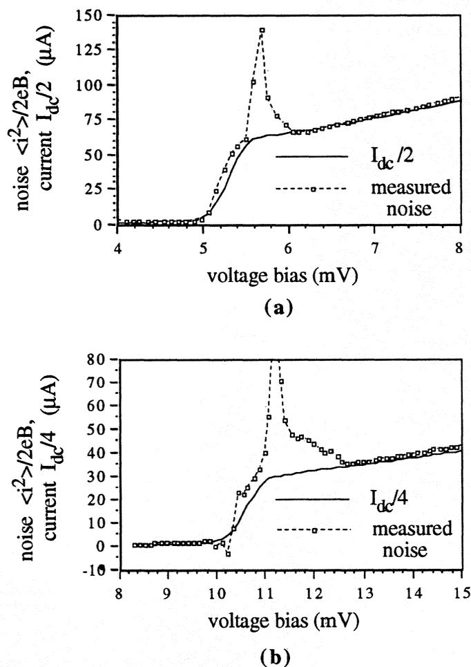
**Figure 4** Measured noise in series arrays of SIS junctions with no incident rf power. (a) is a two junction array and (b) is a four junction array. Also plotted is the dc IV curve with the current scaled down by the number of junctions in the array.
