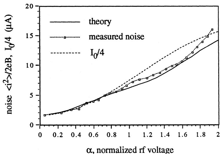
**Figure 8** Photon induced noise in a four junction series array as a function of normalized rf voltage. The array was biased on its first photon step at 9.87 mV. Also plotted is the measured dc current divided by the number of junctions in the array, for comparison to shot noise.
