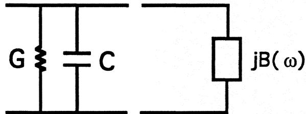
Fig. 7 The circuit model of a Josephson junction with an integrated tuning element. The  $G$  and  $C$  are the junction parasitic conductance and capacitance, and  $B(\omega)$  is susceptance of the tuning element.
