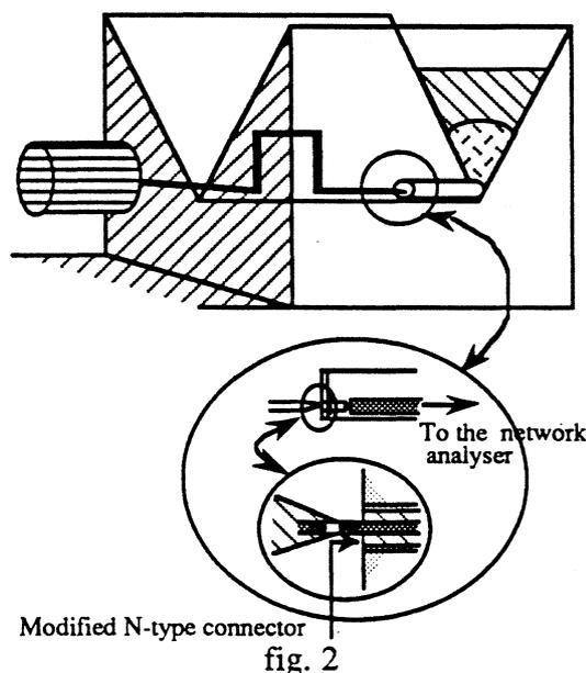
To measure the thickest whisker antenna's impedance it was necessary to make a simple 50Ω transformer to dimensionally match the N-type connector to the 13mm diameter scaled whisker. The signal could then be launched directly into the whisker antenna. The whisker
