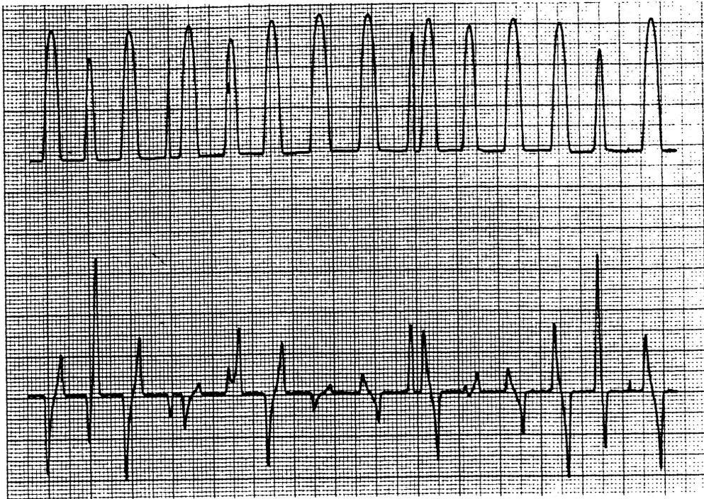
Figure 3c. Demodulated response of slotline photoinductor (chip 1) at 5.32 K, measured on a different run as data in Fig. 3a. Horizontal scale is 50  $\mu$ A/division, vertical scale 0.2  $\mu$ V r.m.s./division.
