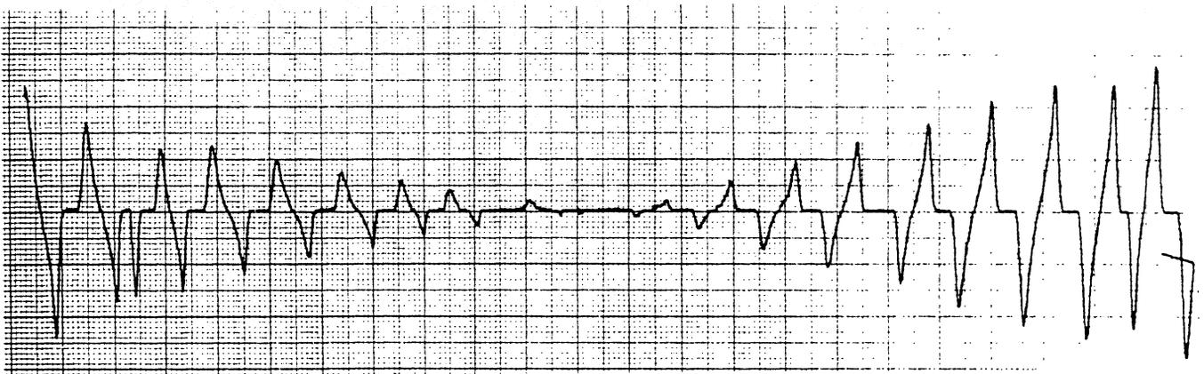
Figure 4. Response to chopped far-IR laser radiation for slotline photoinductor (chip 1). The 404 GHz data was taken at a fixed bias point on the  $V-\Phi$  curve, tweaking  $I_\phi$  so as to hold  $V_{sq}$  fixed.
