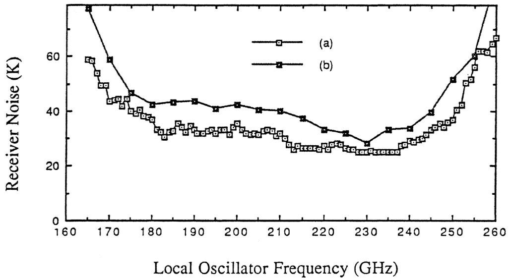
Figure 6. The receiver noise is plotted as a function of LO frequency for two different IFs:
