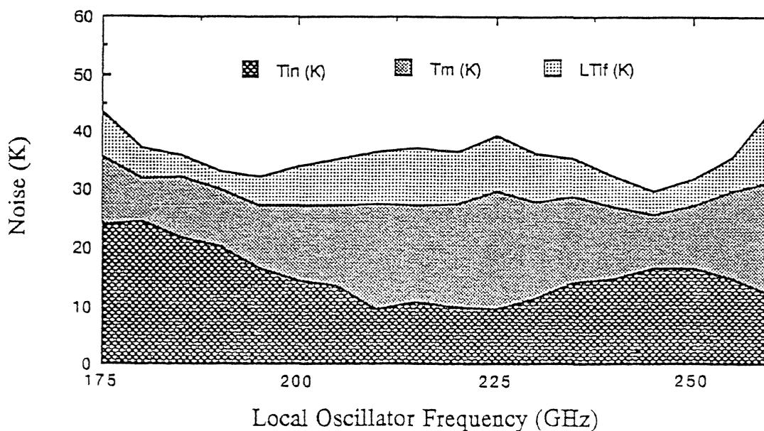
Figure 4. A breakdown of receiver noise into its three components: input loss noise,  $T_{in}$  (K), mixer noise,  $T_m$  (K), and multiplied IF noise,  $LT_{if}$  (K) is plotted as a function of LO frequency.
