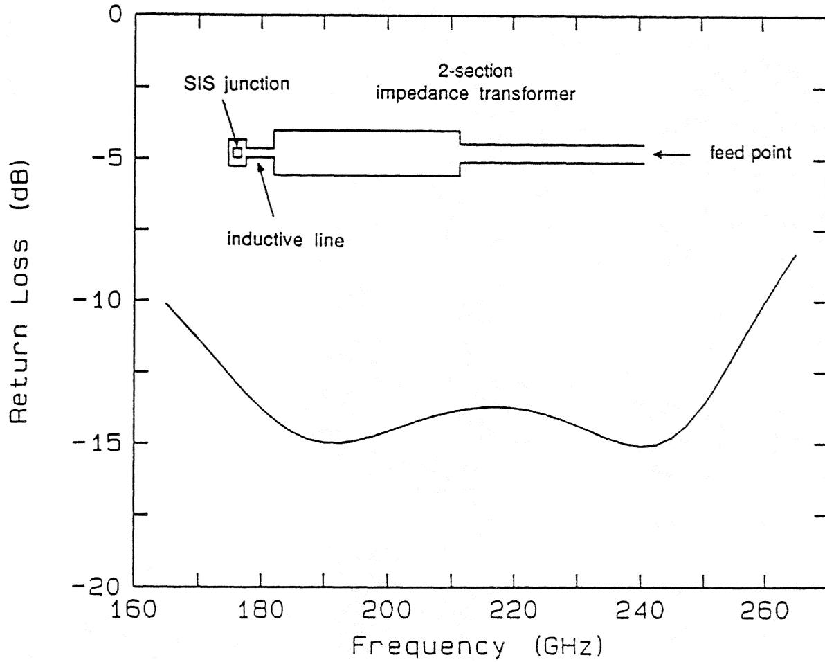
Figure 2. Layout of the integrated microstripline tuning structure showing the SIS junction, the inductive line and the two step impedance transformer. Also shown is the calculated return loss across the signal frequency band.
