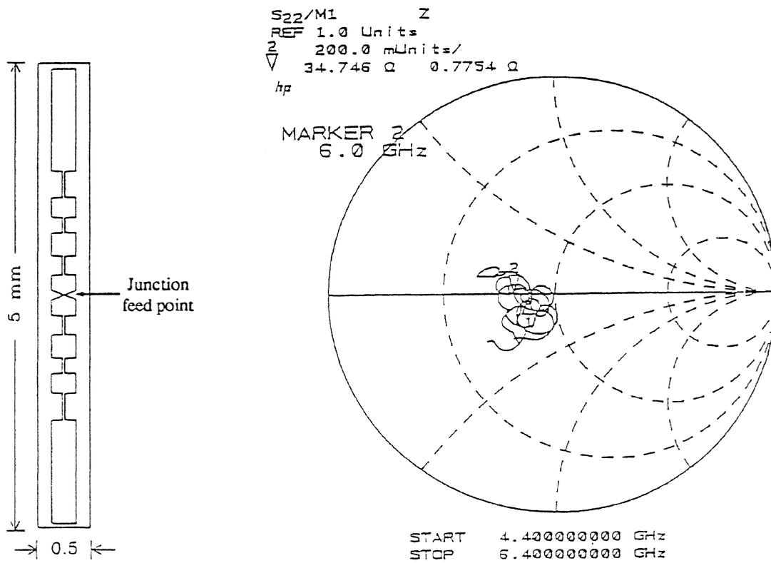
Figure 1b. Suspended substrate filter layout, and the locus of the junction feed point impedance.
