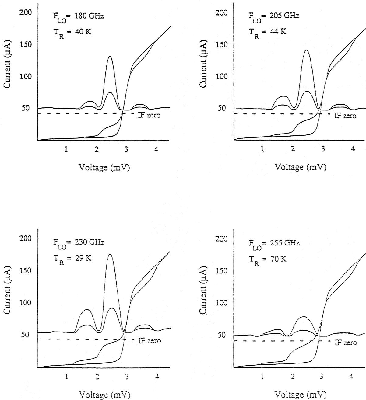
Figure 5. Current-voltage characteristics, pumped and unpumped, are given for four different LO frequencies. Also shown is the receiver output in response to hot (295 K) and cold (77 K) input loads.
