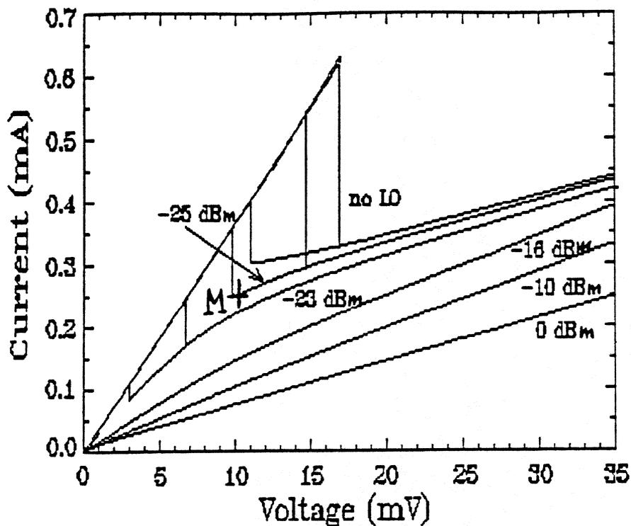
Fig. 4. IV-curves under LO power for sample No. 1.
