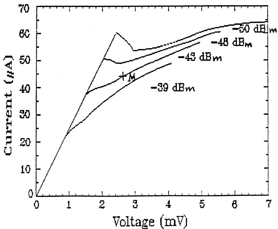
Fig. 5. IV-curves under LO power for sample No. 2.
