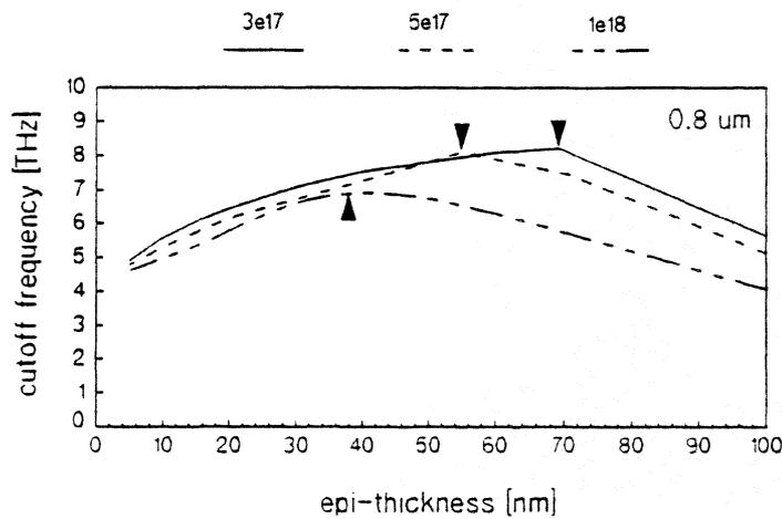
Fig.2: Standard cut-off frequency for 0.8  $\mu\text{m}$  anode diameter
