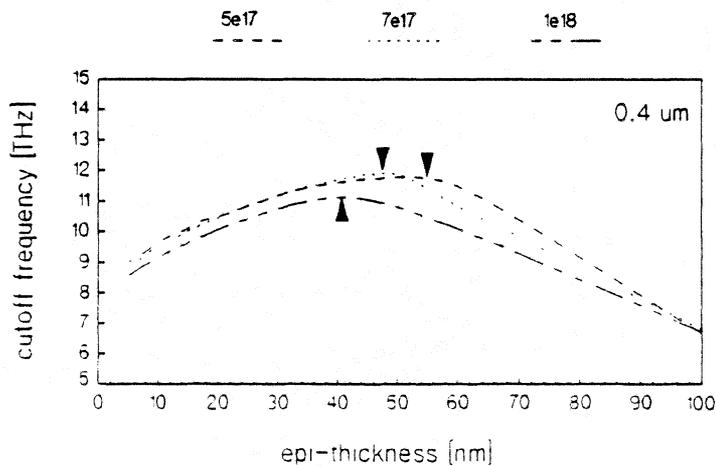
Fig.3: Standard cut-off frequency for 0.4  $\mu\text{m}$  anode diameter
