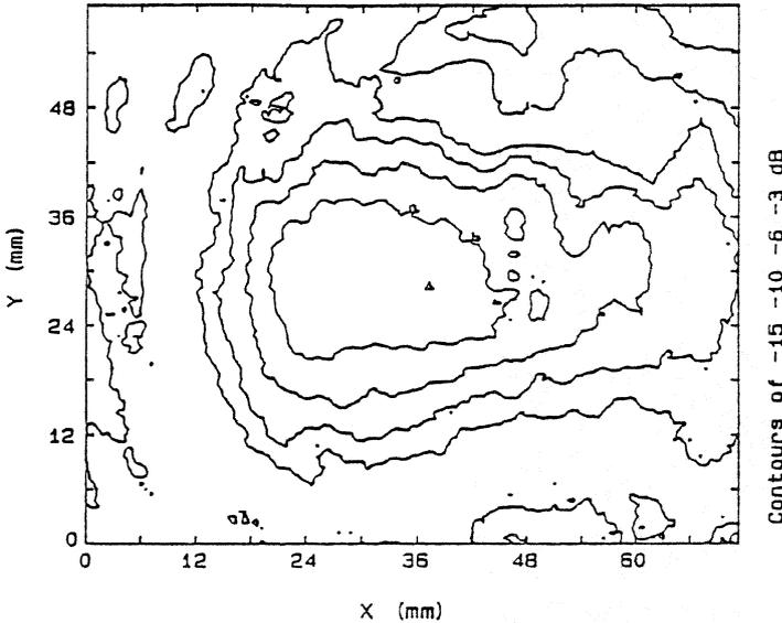
Fig. 9 Near Field Amplitude Data at 254 GHz of Twin Dipole Receiver on Ellipsoidal Lens
