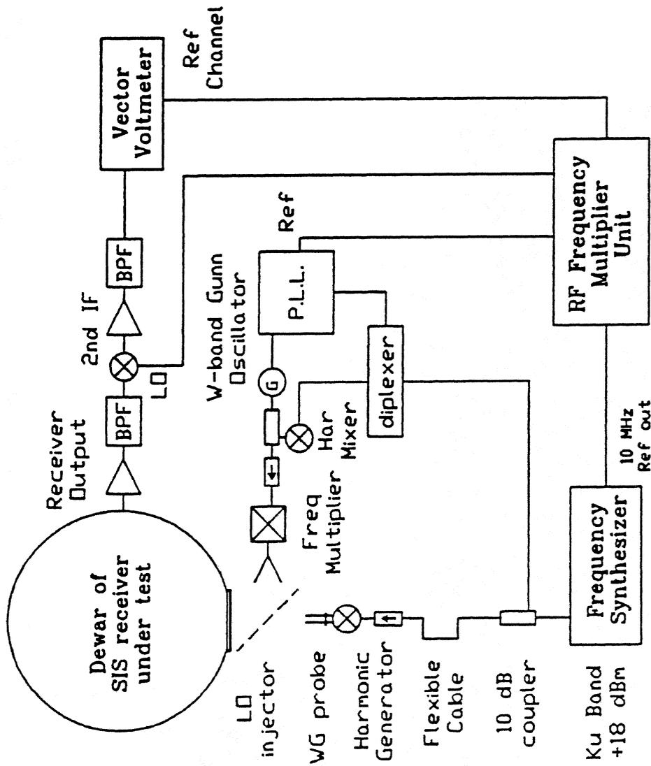
Fig. 1 Block Diagram of Near Field System
