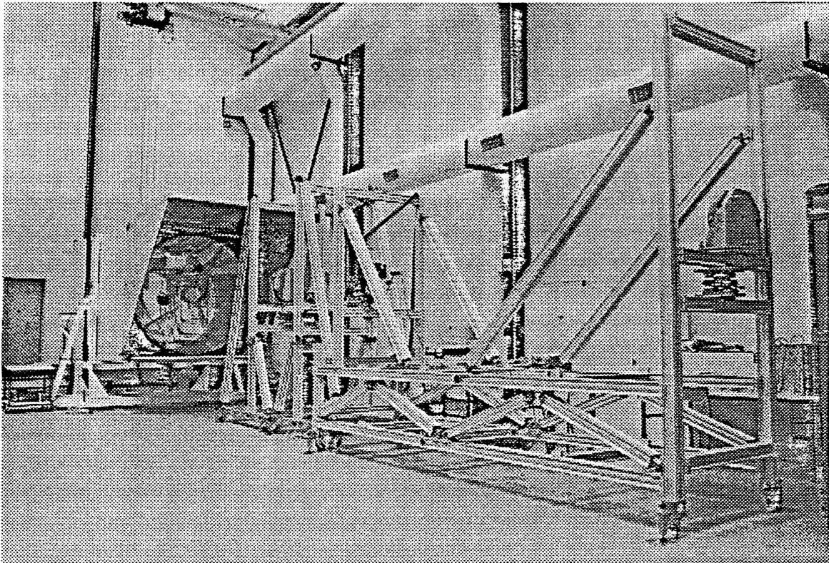
*Figure 6' : PRONAOS telescope under alignment procedure*
