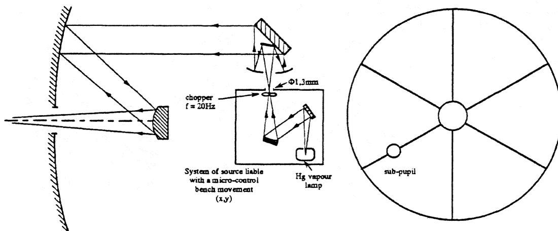
Figure 7: Mounting of the collimated beam
