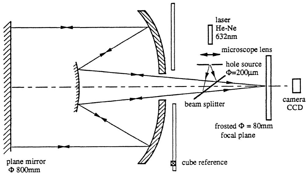
Figure 6: Autocollimation schema
