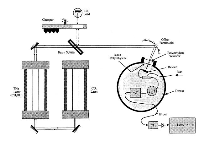
Figure 5: Optical layout of the noise temperature measurements.
