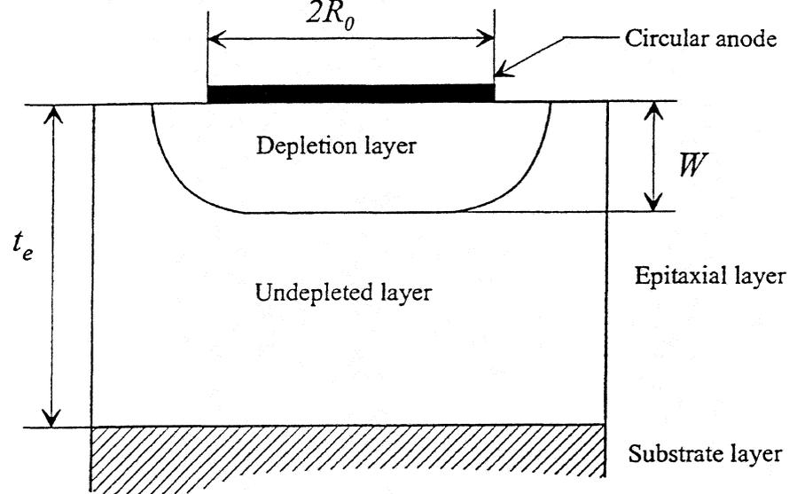
Figure 1: Schematic of the Schottky varactor.
