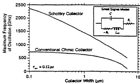
Fig. 2: Comparison of a conventional RTD to a Schottky-Collector RTD using measured values of  $R_n$  and  $C$  from the 5 ML AlAs/In<sub>0.53</sub>Ga<sub>0.47</sub>As SRTD, inclusive of the effects of  $\tau_{qw}$ . The inset shows the small signal equivalent circuit model of an RTD biased in the negative differential resistance region.
