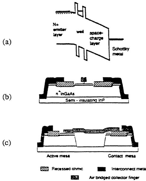
Fig. 1: (a) Band diagram, (b) and (c) perpendicular cross sections of a submicron AlAs/In<sub>0.53</sub>Ga<sub>0.47</sub>As SRTD.
