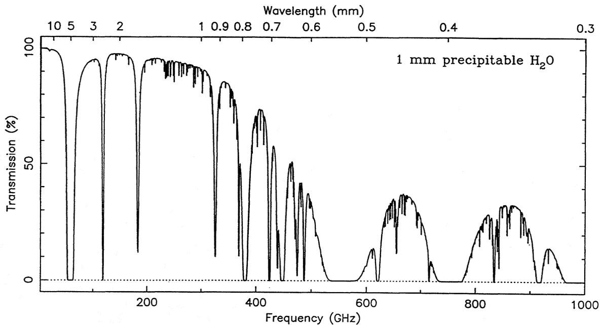
Figure 2. Model of the atmospheric transmission<sup>10</sup> at a 4000 m altitude and for 1 mm precipitable H<sub>2</sub>O.
