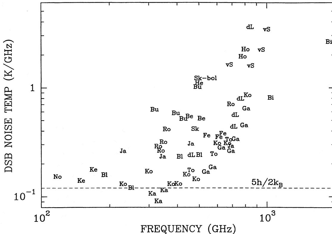
Figure 5. Compiled SSB noise temperatures for SIS receivers<sup>14</sup>.
