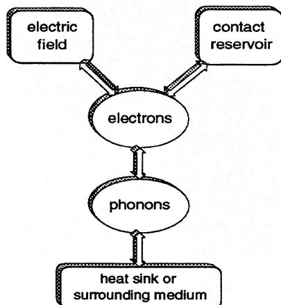
Figure 1: Energy picture of the Gunn device.
