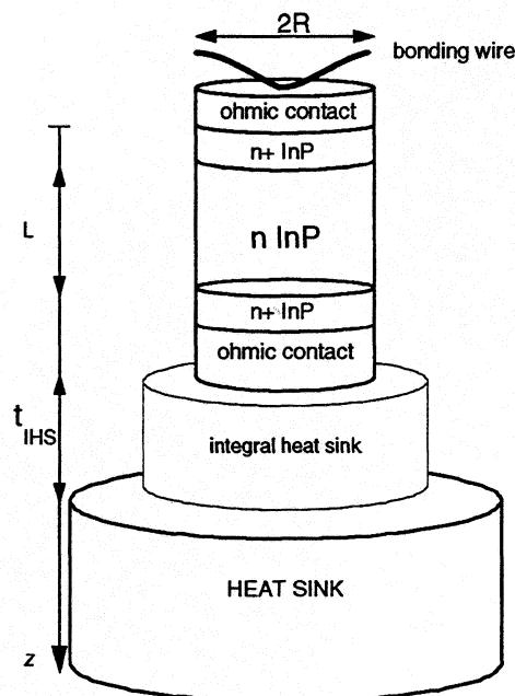
Figure 2: Gunn device on a heat sink.
