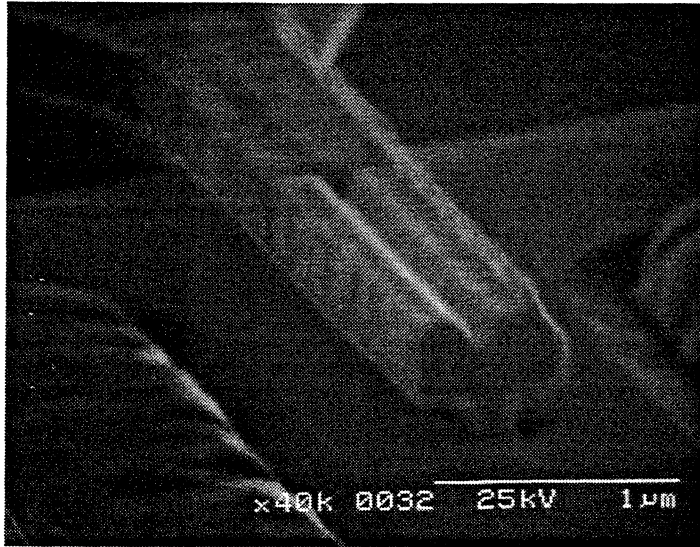
Fig 2. SEM photograph of a T-anode Schottky diode fabricated in the JPL Micro Devices Laboratory (MDL).
