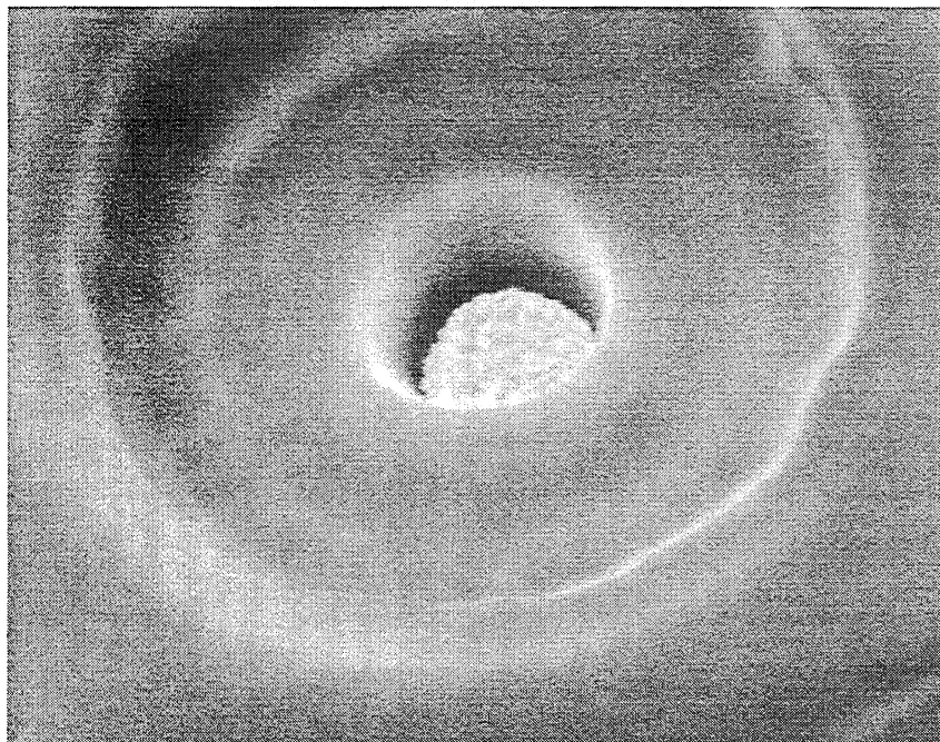
Fig. 8. Anode after buffered HF etch and platinum deposition with thin gold overplate (15° Tilt)
