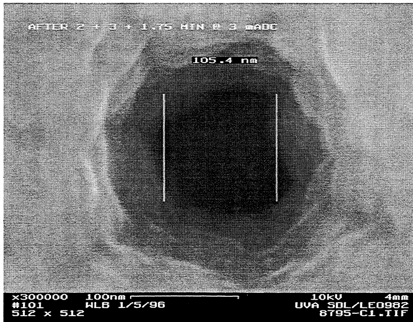
Fig. 5. Anode pattern after electroplate window shrink (EWS)
