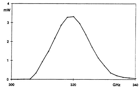
Figure 14 - Performance computed with finite element analysis and harmonic balance of the second iteration design of the 320 GHz MMIC doubler. Input power is 15 mW at 160 GHz.
