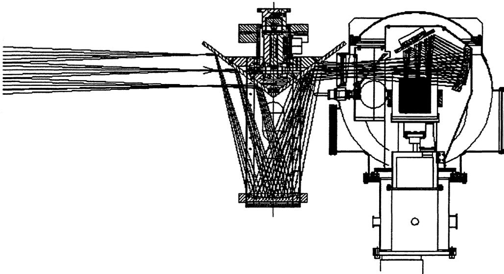
Fig. 1 : Layout of the 230 Hz SIS multibeam receiver. Although only nine beams are indicated the occupied field of view corresponds to a 4x4 field covered with beams separated by 2 FWHM . The horns of the mixers are orientated perpendicular to the plane of view.
