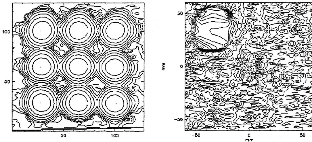
Fig 3. : Left: Measured amplitude pattern of the assembled receiver optics in 5 dB steps.
