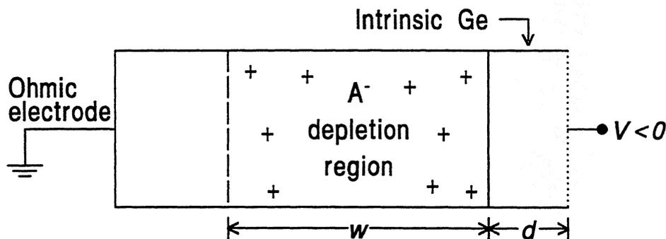
Figure 1: Schematic of a Ge:Ga BIB.
