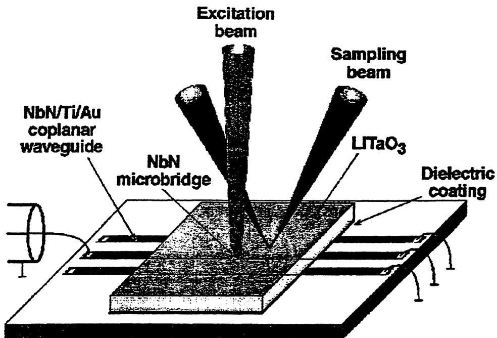
**Fig.4** Electro-optic sampling is performed by covering the NbN microbridge with LiTaO<sub>3</sub> crystal.
