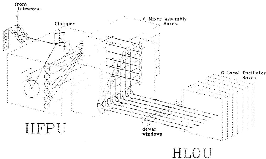
Figure 5. Perspective view showing the LO beam disposition
