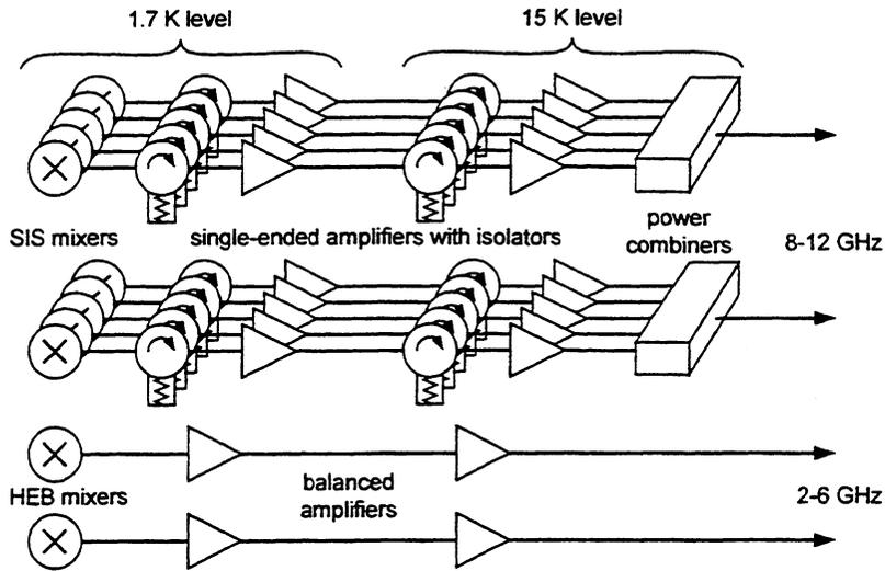
Figure 6. Block diagram of IF pre-amplification scheme.
