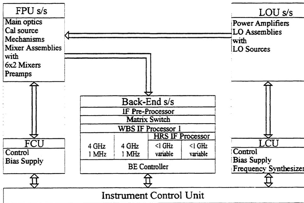
Figure 1. Block diagram of the *HIFI* instrument
