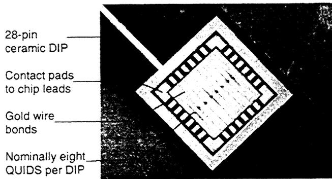
Figure 2: Devices mounted on ceramic chip carrier for thermal lifetime tests.
