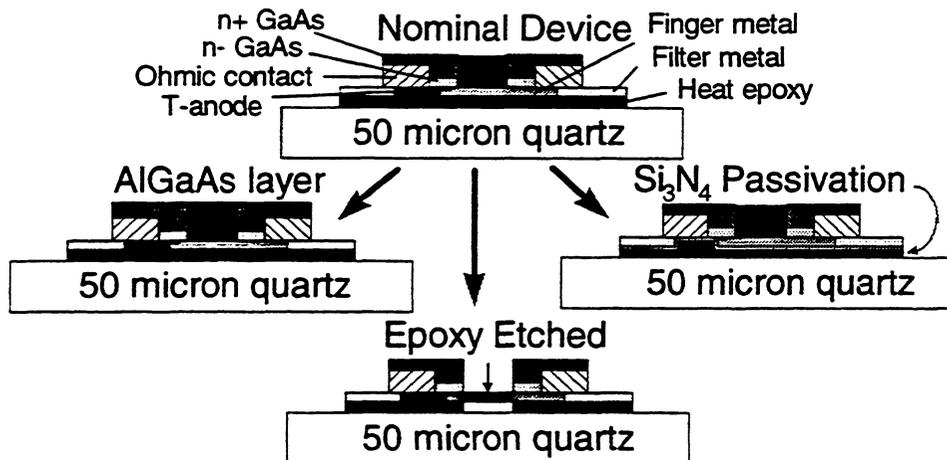
Figure 4: Device Processing Variations: (1) AlGaAs etch-stop layer, (2) epoxy-etched channel, (3) Si<sub>3</sub>N<sub>4</sub> passivation. (Figures not drawn to scale)
