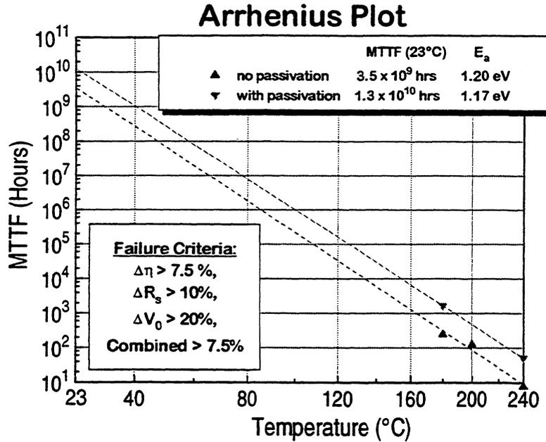
Figure 11: Arrhenius Plot for devices with and without  $\text{Si}_3\text{N}_4$  passivation layer. Note that the failure criteria was tightened to obtain 50% sample failure from the nitride passivated devices.
