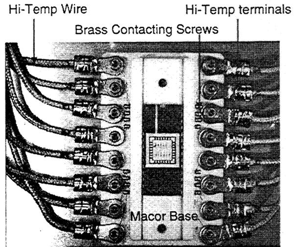
Figure 3: Macor-based solder-less mounting fixture rated to 340°C.
