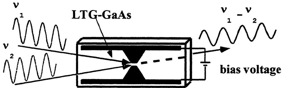
Fig.1. Schematic diagram of a photoconductive antenna device.
