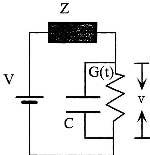
Fig.2. Equivalent circuit of the photoconductive antenna device.
