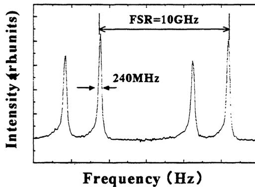
Fig.5. Spectral linewidth measured using a scanning Fabry-Perot interferometer.
