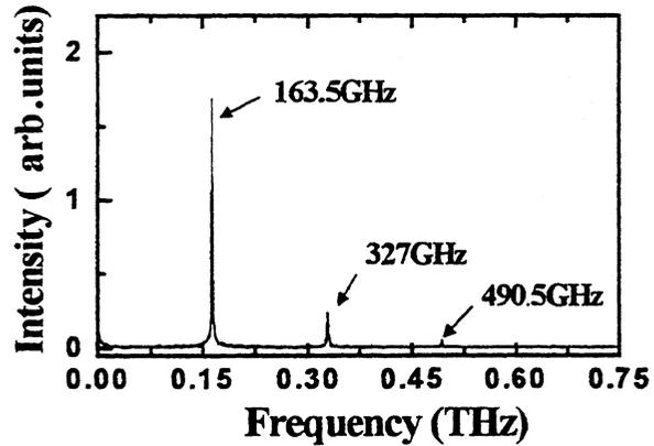
Fig.8. FFT spectrum of the interferogram
