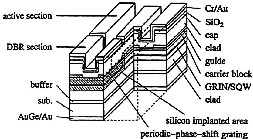
Fig.3. Schematic diagram of a two-longitudinal-mode DBR LD.
