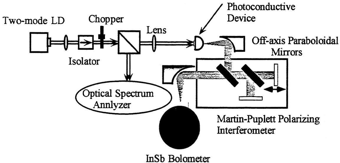
Fig.6. The experimental set-up to generate coherent cw-THz radiation and to measure the radiation properties.
