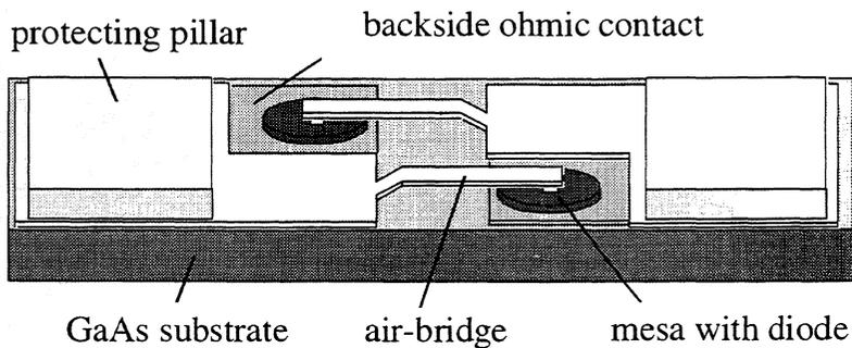
Figure 2: Geometrical structure of an APQVD chip.
