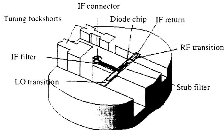
Figure 1: Sketch of the 220 GHz mixer block.
