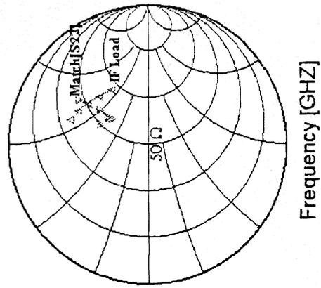
Fig. 7 A 4-8 GHz IF matching network which transforms a 50 Ohm input impedance to the required IF load impedance given the condition,  $S_{11}(\text{RF}) = -3\text{dB}$ . Since it is physically impossible to provide a negative capacitance, a good impedance match can only be provided over a limited (octave) of bandwidth.
