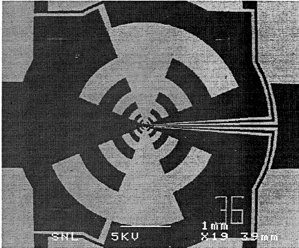
Figure 7. View of a chip with a planar log-periodic antenna and the microbolometer in the focus of the antenna designed for device tests at 100-1000 GHz.
