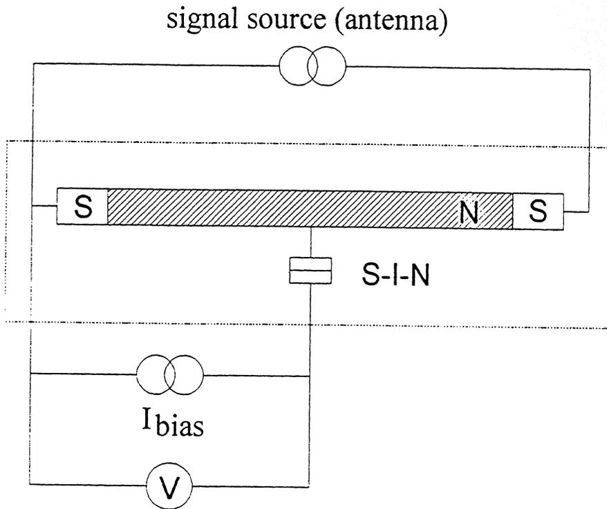
Figure 6. Schematic of the microbolometer: the SIN junction is biased at a small constant current. A junction voltage depends on the smearing of the IV-curve which is used to measure the electron temperature in the normal metal absorber (hatched).
