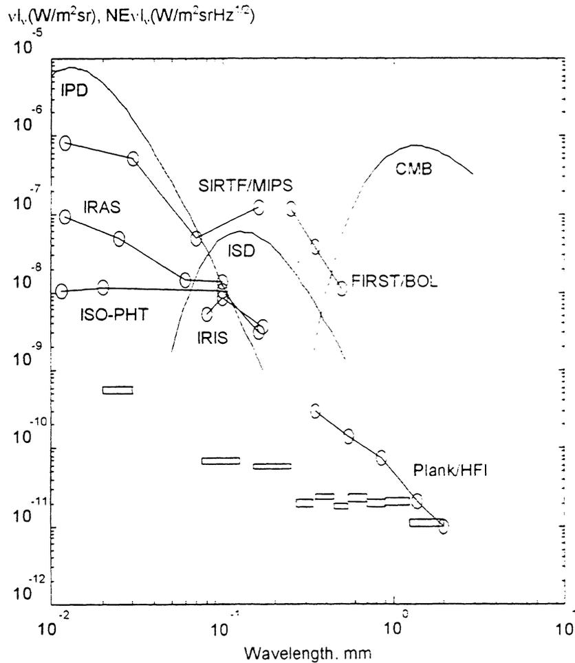
Figure 3. The sensitivity related to brightness of extended sources. Rectangles - the Submillimetre Project, circles - other projects.  $NE \nu I_\nu$  - noise equivalent brightness with  $S/N=1$ . The brightness of sources given for comparison: CMB - cosmic microwave background, ISD - interstellar dust emission, IPD - interplanetary dust emission.
