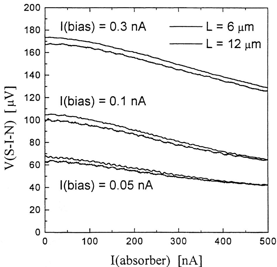
Figure 9. The junction voltage  $V$  at constant bias current  $I_{\text{bias}}$  through the junction as a function of the signal current  $I_{\text{ABS}}$  for two devices with different absorber length 6  $\mu m$  and 12  $\mu m$  at  $T=30mK$ .
