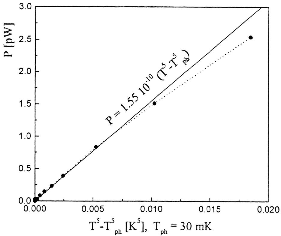
Figure 10. Power dissipated in the absorber vs.  $(T^5 - T_{ph}^5)$  where  $T$  is temperature of electrons deduced from measurements  $V(I_{bias}, T)$  and  $T_{ph}=30 \text{ mK}$  is temperature of the lattice (measured temperature of the sample holder). Linear fit corresponds to the relation (2).
