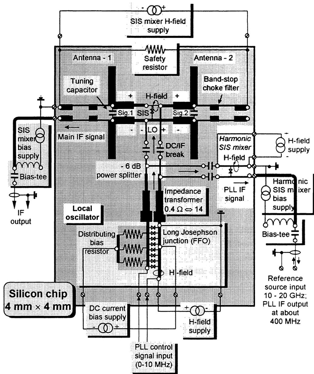
Fig. 2. Simplified equivalent diagram of external supplies and connections necessary to operate the chip of Superconducting PLL Receiver.
