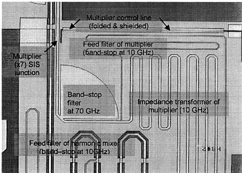
Fig. 5. Partial view of the integrated receiver chip. Folded striplines are feed filters at 10 GHz and 70 GHz used for the SIS multiplier and for the harmonic mixer. Field of view is about 900 x 600 micrometers.
