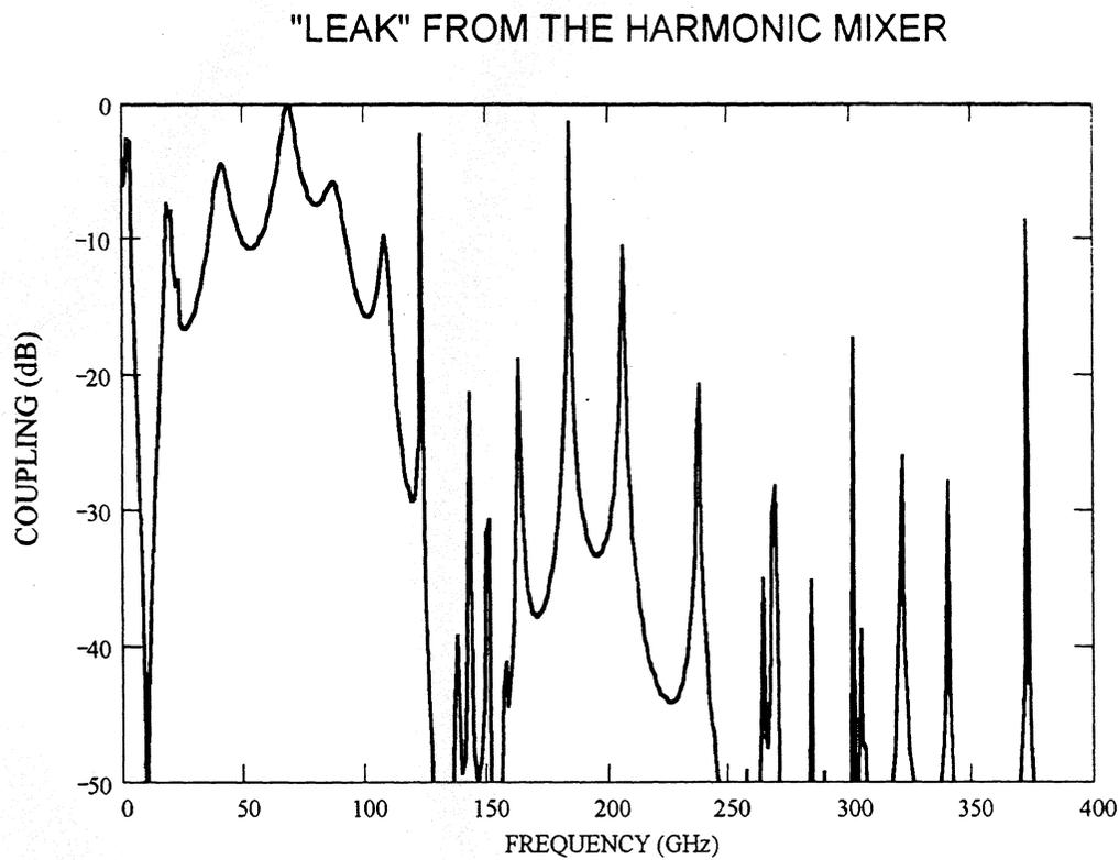
Fig. 6. Reflection loss at the harmonic mixer towards its IF port and towards the SIS multiplier (if used). Coupling to FFO that is, by definition, strong *excluded* from this calculation.
