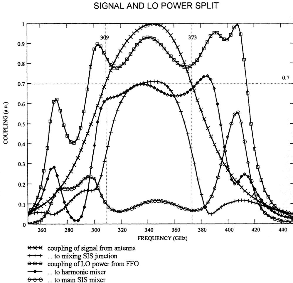
Fig. 4. Example of calculated distribution of signal (x's and +'s) and local oscillator power (box's and dimond's) in the PLL receiver circuitry. Fraction of LO power used by main SIS mixer presented at the bottom by o's. The data calculated for central frequency of 350 GHz.
