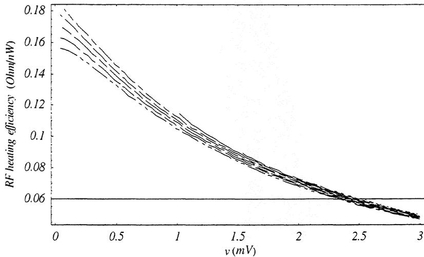
Fig. 4 Calculated LO/RF heating efficiency along the self-consistently calculated IV curves from Fig.3. The curves are obtained for 350nW (bottom curve),310nW, 270nW, 230nW and 190nW (top curve reaching down to zero bias voltage) LO power. There are two more IV curves starting at higher bias voltages for 150nW and 110nW.
