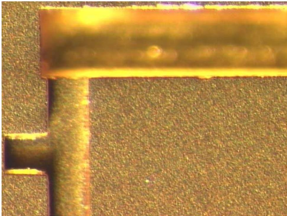
*Fig. 1: Two views of the 585 GHz split-block mixer, top: the flared horn, waveguide and microstrip channel, and bottom: a view of the waveguide, backshort and part of the channel. Note the extremely sharp features. Also, the bottom of the channel is the metallized silicon surface. The microstrip channel width is 120  $\mu\text{m}$ .*
