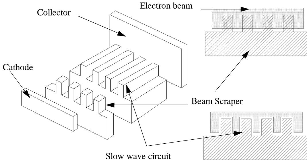
**Figure 1. Basic configuration of the existing BWO design**
