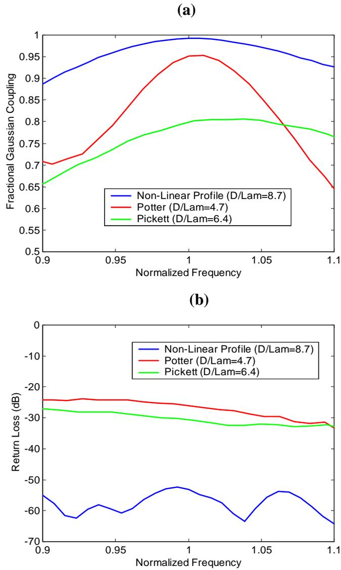
**Figure 4. Comparison of Gaussian coupling and return loss for non-linear taper profile and other published designs. (a) Fractional Gaussian coupling versus normalized frequency. (b) Return loss versus normalized frequency.**
