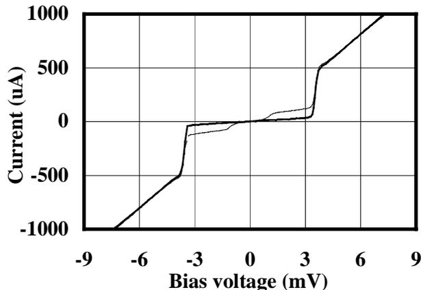
Fig. 1. Current-Voltage characteristic of the NbTiN/AlN/Nb junction with (thinner line) and without radiation at 1130 GHz. Critical Josephson current density is about 30 KA/cm<sup>2</sup>.
