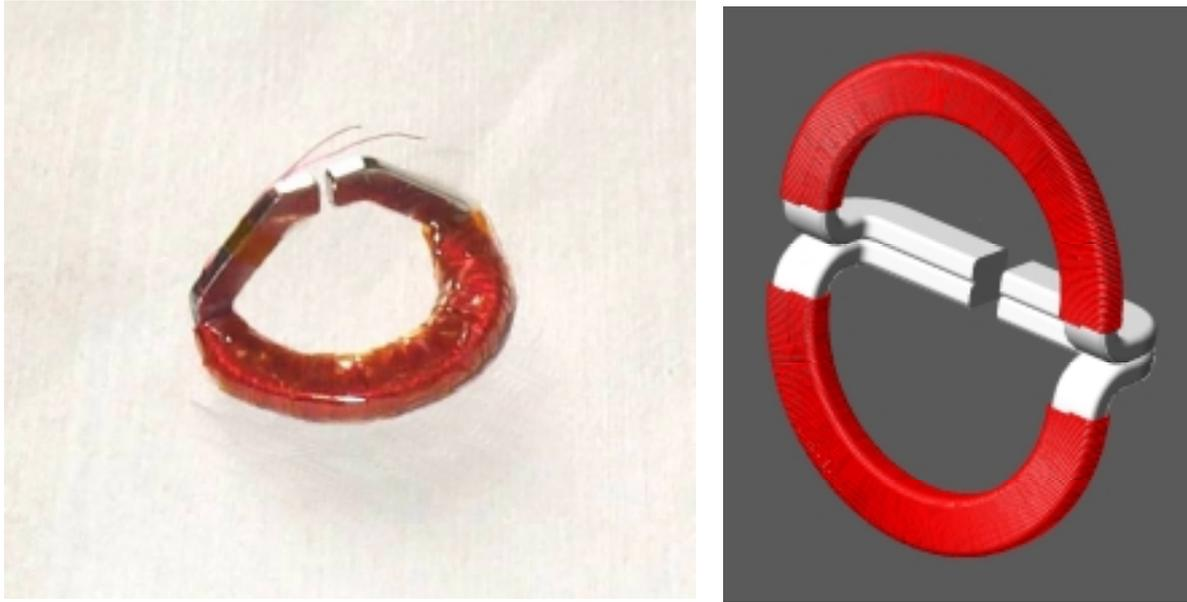
Figure 8. One half of the cryoperm electromagnet designed for Band 1 (1100 turns); artist's view.
