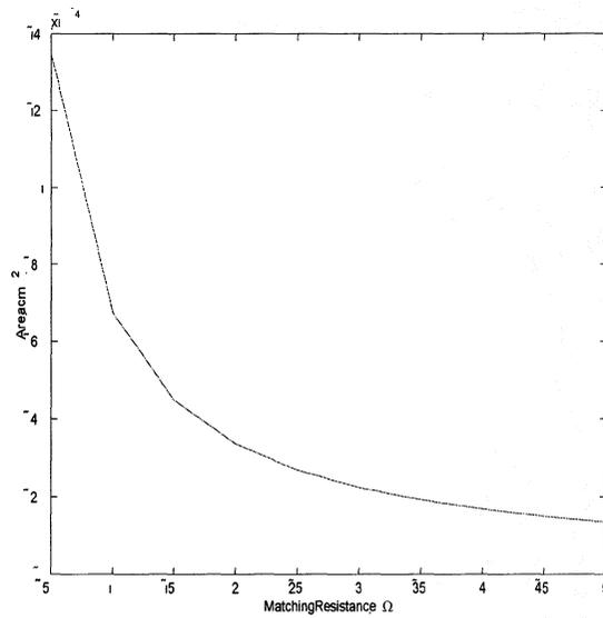
Figure 6: Small Signal Device Area  $J_{DC} = 1000A/cm^2$
