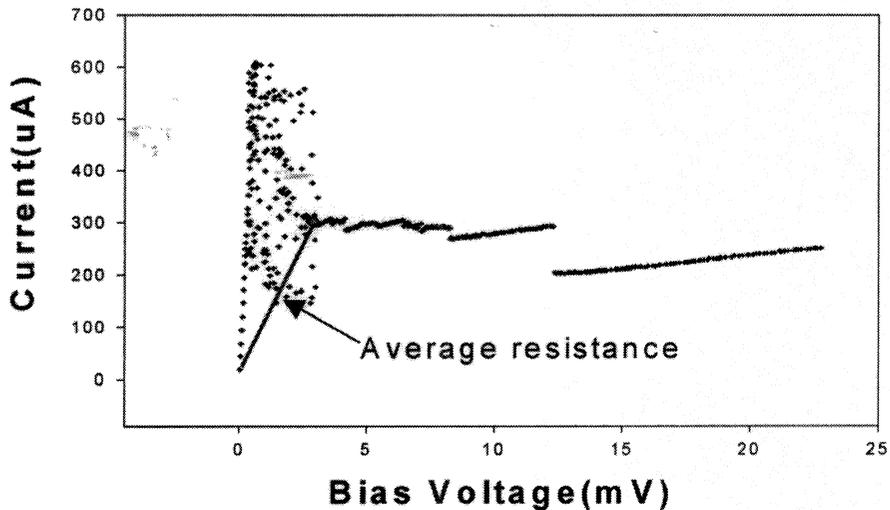
Fig. 7: Average resistance of HEB at the operating point during ANA measurement
