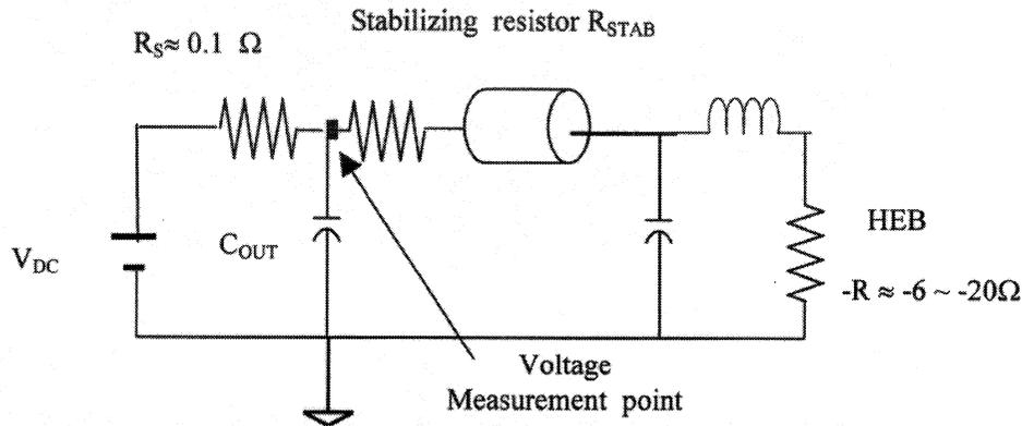
Fig. 3: HEB measurement circuit diagram after inserting stabilizing resistor
