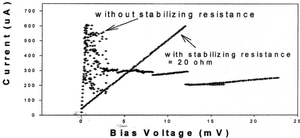
Fig. 4: I – V Characteristics of HEB Device with stabilizing resistor
