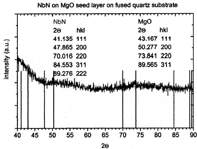
Fig.1.1.:  $\theta/2\theta$  scan of an NbN/MgO bilayer on a fused quartz substrate
