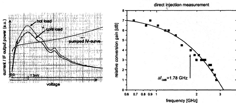
*Fig.5.1.: Pumped I(V)-curve and conversion curves of an NbN/MgO HEB; IF bandwidth determined by double local oscillator injection.*
