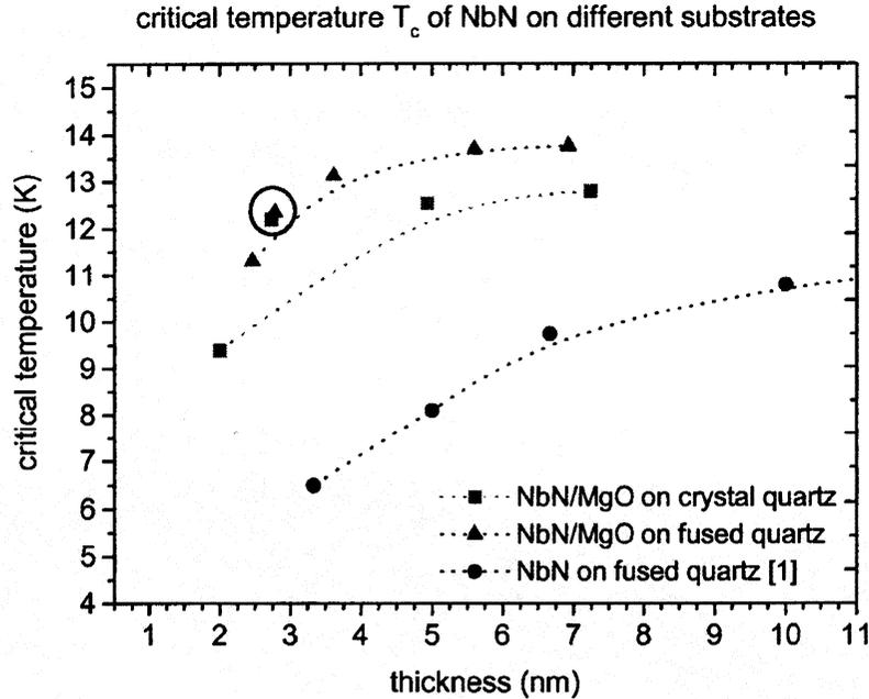
Fig.3.2.: Critical temperature vs. film thickness of NbN/MgO bilayers compared to NbN on fused quartz substrates.
