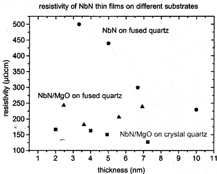
*Fig.3.1.: Resistivity vs. NbN film thickness of NbN/MgO bilayers compared to NbN on fused quartz substrates.*
