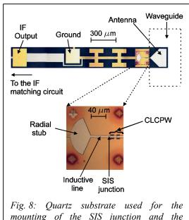
mounting of the SIS junction and the integrated tuning structure
