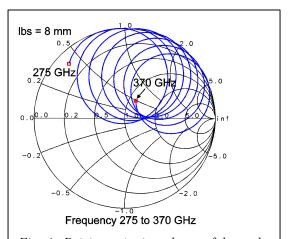
Fig. 4: Driving point impedance of the probe for the mixer geometry shown in Figs.3 and 8: The circular backshort is located at a distance  $l_{bs}$ =8mm away from the antenna plane. The Smith chart is normalised to 50 **W**.
