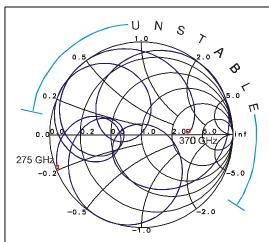
Fig. 5: Series inductive tuning with twosection 1/4 transformer. Impedance seen by the junction. Note that the reactive termination used for image rejection lies, in some cases, in the "unstable" region. The Smith chart is normalised to  $Z_S=R_n$
