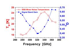
Fig. 9: Calculated SSB mixer noise temperature and coupled mixer gain in the signal band  $G_S$  (linear scale) in the 275-370 GHz frequency band.
