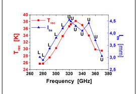
Fig. 10: Calculated SSB receiver noise temperature  $T_{rec}$  and backshort in the 275-370 GHz frequency band, in LSB (L) or USB (U).
