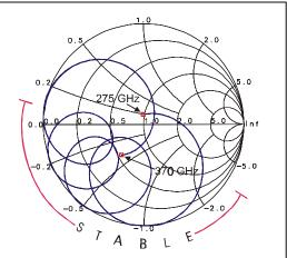
Fig. 6: Parallel inductive tuning with singlesection 1/4 transformer. Impedance seen by the junction. The reactive termination used for image rejection is always within the "stable" region. Here the backshort distance is 4.2 mm, appropriate for USB operation at 320 GHz.
