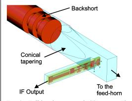
Fig. 3: Full height waveguide SSB mixer. The circular section backshort is used for image rejection.
