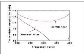
Fig. 2: Amplitude of the transmission coefficient of six sections <sup>2</sup>Hammer<sup>2</sup> type and normal type filter as a function of frequency.
