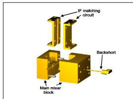
Fig. 11: Mixer block configuration: the two main parts of the mixer used for the SIS junction mounting are shown together with the circular section backshort and the shielded microstrip used as IF matching transformer.
