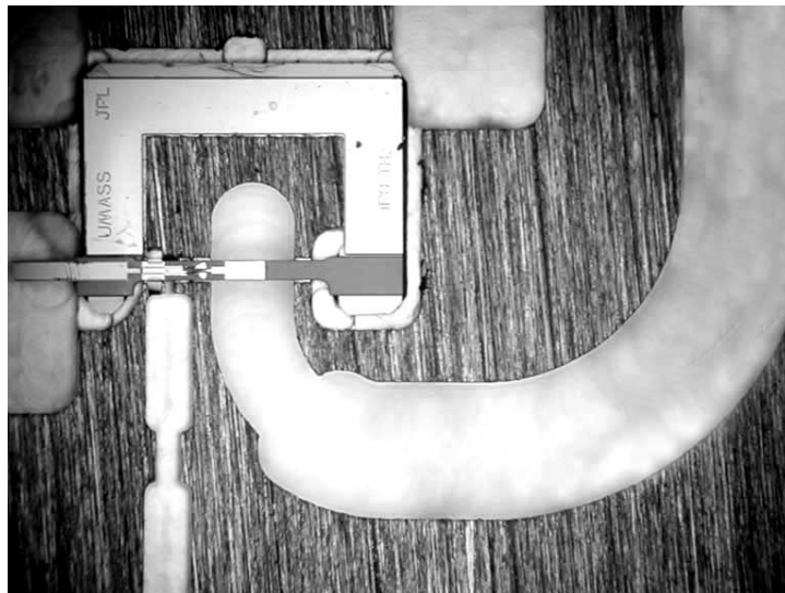
Figure 9. Overall view of the 1 THz tripler showing the complete frame, bias beam lead on the left, and the wrap-around input waveguide on the right.
