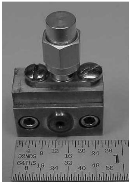
Fig. 3: Assembled MOMED tripler. The outer block dimensions are: HxWxL = 16 x 20 x 10 mm (without the SMA connector).
