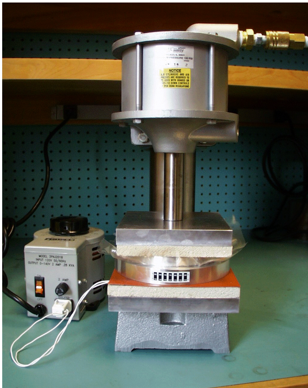
Figure 9. Photograph of the assembled window press. The Variac and heating pad are used to increase the temperature of the jig and so decrease the curing time of the epoxy. Note the thin film thermometer on the lower half of the jig.
