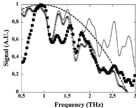
Fig.7. Direct response of the spiral antenna integrated NbN HEB mixer (squares), calculated transmission of the atmosphere between the FTS and the cryostat (solid), simplified parabolic spiral antenna response (dashed) and the interpolation of the parabola with the atmosphere transmission curve (crosses).
