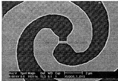
Fig. 1. SEM micrograph of an NbAu mixer. The NbAu bridge is located between the arms of the spiral antenna. The Au cooling pads are part of the antenna. The bar represents 2  $\mu\text{m}$ .
