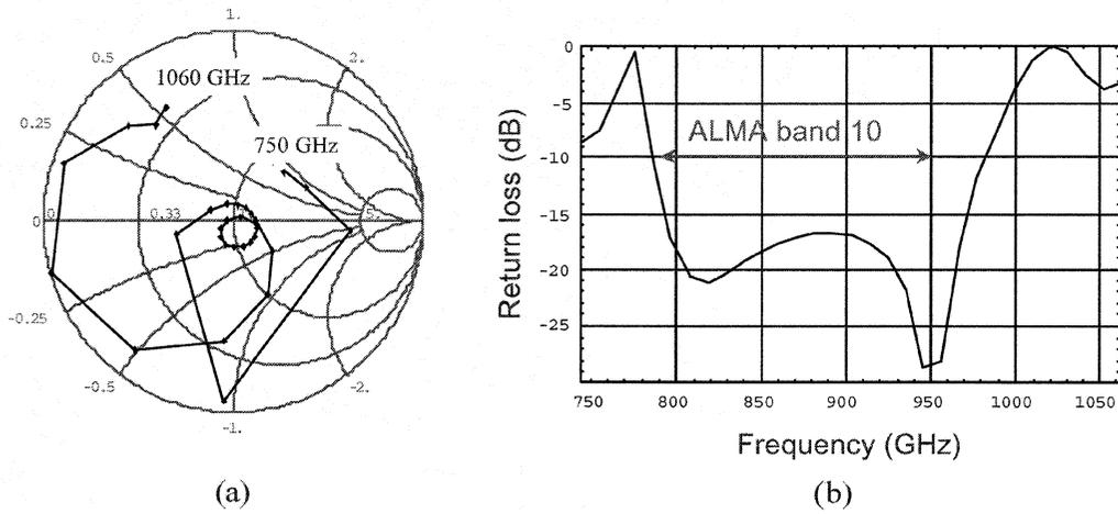
Fig. 2. (a) Calculated feed-point impedance normalized to  $60 \Omega$ . (b) Return loss characteristics between feed-point and  $60 \Omega$ .
