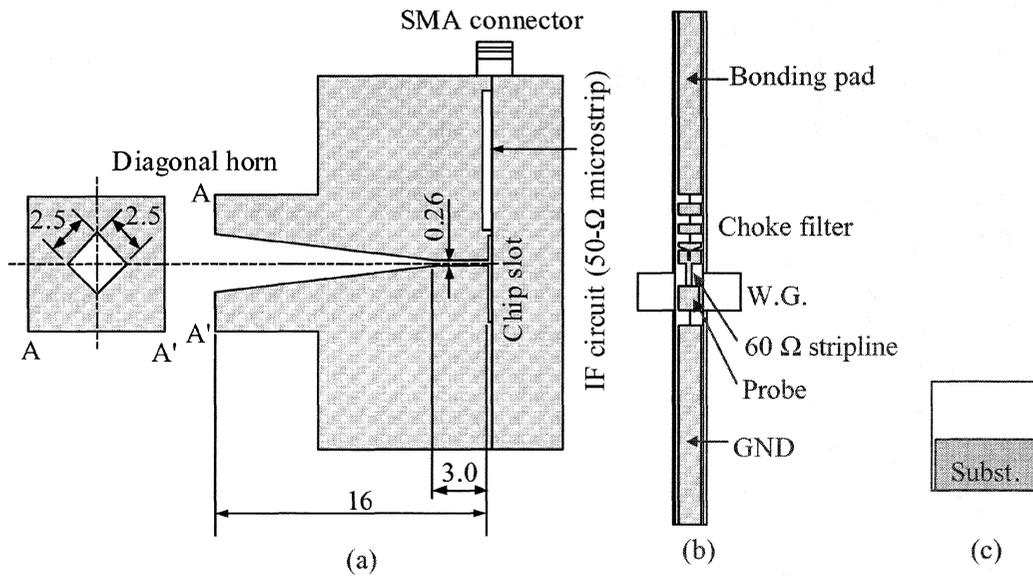
Fig. 1. Mixer mount layout showing diagonal horn section and mixer back piece. (b) View of chip slot from side of back piece. Waveguide is 0.1 × 0.26 mm, substrate is 0.07 × 1.4 × 0.032 mm. (c) Sectional view of chip slot, which is 0.073 × 0.073 mm.
