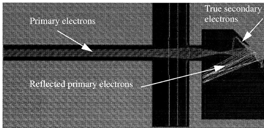
**Figure 10. Simulation of sheet electron beam with single stage depressed collector. Primary electrons, reflected primary electrons, and true secondary electrons are indicated. Simulation is at 5,000 Volts, 30 mA.**
