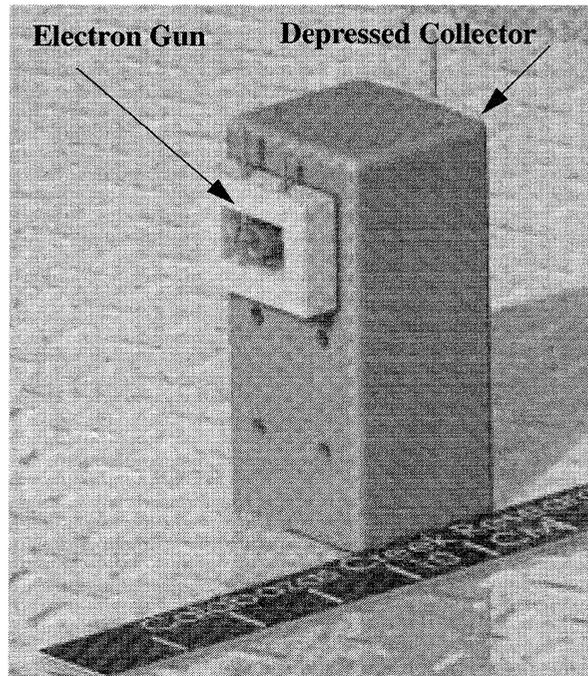
**Figure 11. 600-700 GHz Beam Line Assembly.**
