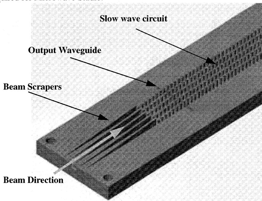
**Figure 1. Layout of BWO circuit. The beam scrapers carves grooves in the rectangular electron beam for the slow wave structures downstream. The RF power is extracted through the base into rectangular waveguide.**
