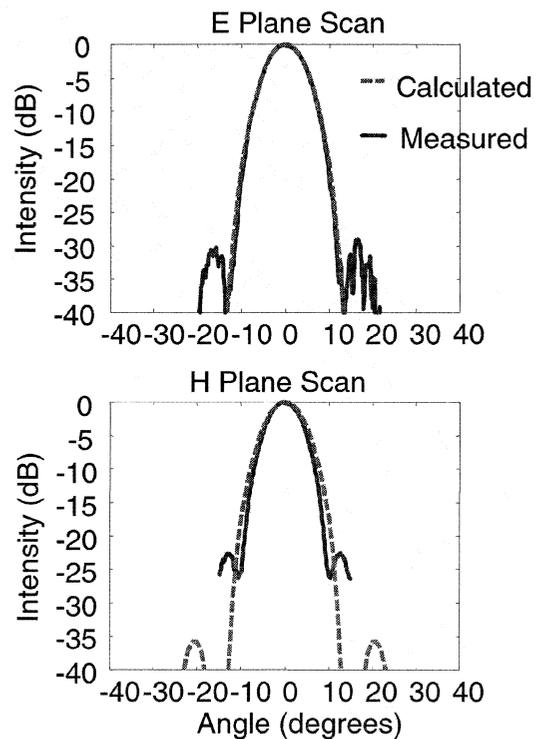
Figure 9. Measured performance of scaled output horn
