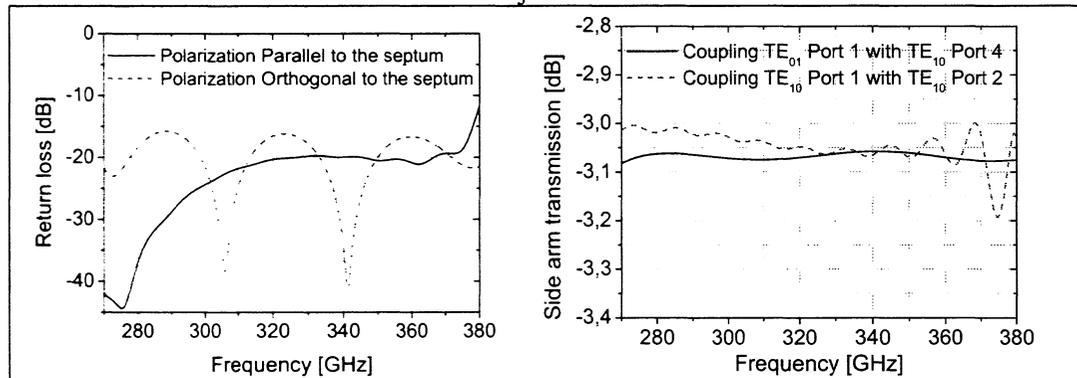
Fig.(4): Result of simulations of the 5-port device illustrated in Fig.(2). *Left*): Amplitude of reflection coefficient at the input (Port 1) for polarization parallel, and orthogonal to the septum. *Right*): Solid line: Coupling amplitude between fundamental mode at Port 1 with E-field orthogonal to the septum and fundamental mode at Port 4 (or 5). Dashed line: Coupling amplitude between fundamental mode at Port 1 with E-field parallel to the septum and fundamental mode at Port 2 (or 3).
