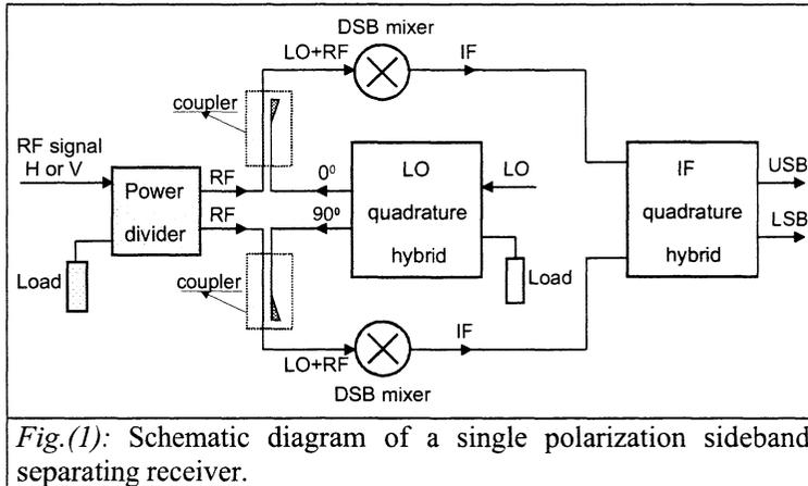
Two  $\lambda_g/4$  long shunt guides are used in the 16 dB couplers. The couplers were realized by splitting the blocks on the E-plane; this facilitates their integration with other components. All the elements of the network were designed and tested at IRAM.
