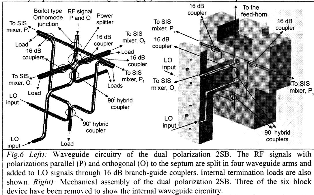
branch-guide couplers, two  $90^\circ$  hybrid couplers as well as the orthomode junction and power splitter. Once assembled, the device will have external dimensions  $40 \times 40 \times 40 \text{ mm}^3$ . A beryllium copper septum (not visible) can be positioned between hollow surfaces of two split-blocks. The blocks can be realized using a standard CNC, except for the slots of the waveguide couplers that require to use spark-erosion technique.
