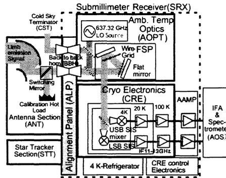
Fig.2 Block diagram of 640 GHz receiver for SMILES.
