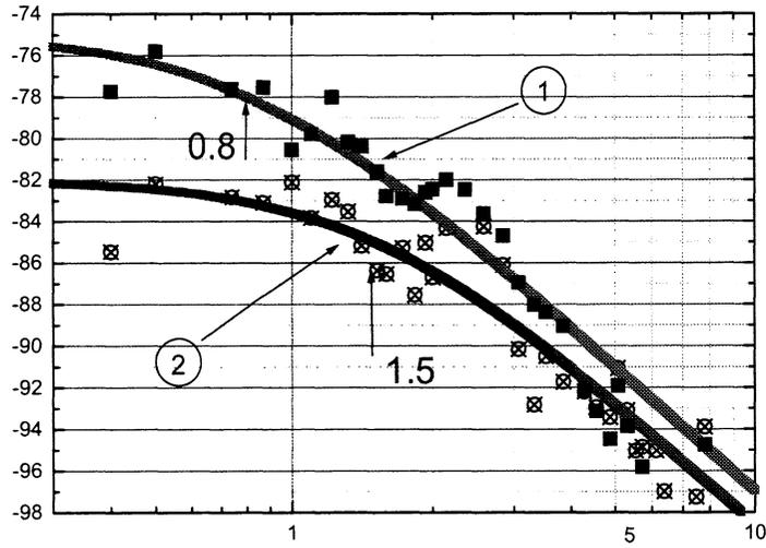
Fig. 3 Output power as a function of IF for 0.13  $\mu\text{m}$  long device based on 3.5 nm thick film. Experimental data are marked by squares (for optimal operating point) and crossed circles (for larger bias voltage).
